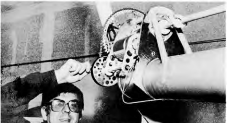
Bob Boucher, consultant for solar cells and electric motor, fits Astro Flight motor. Lower rubber belt cog drives bicycle chain and spocket to give 23:1 reduction to propeller
