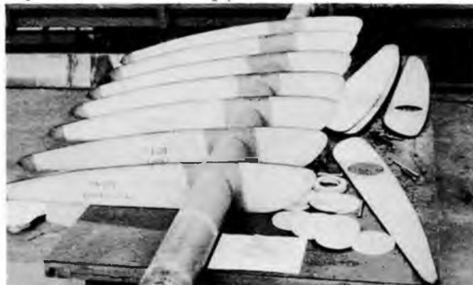
Above: Paul MacCreedy attempts to break the wing! Once flat wing deflected 18ins at tips to support almost half a ton of sand during positive +6G test. Unique flat topped aerofoil allowed upside-down construction. Below: here 1/4 in. expanded polystyrene wing ribs are threaded onto main wing spar.
