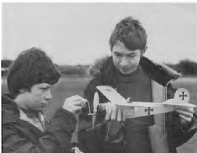
The model needs holding securely while winding, as there is considerable torque from the eight strands of 6mm flat rubber. Give only 30 turns for the first few flights, until the model is trimmed, and the rubber is broken in.
