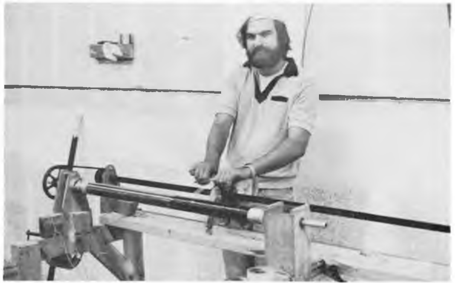
Project manager Ray Morgan wraps carbon fibre tube with heat shrink polypropylene tape. Rear spindle advances tape spool, as front carbon tube rotates
