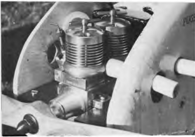
Prototype 7cc Oliver Twin-Major, here installed in Lynn Walter's scaled up 'Scram' vintage model. A production version is, hopefully, in the offing.
