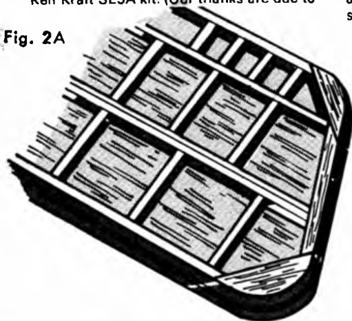
Left: structural modification made to the tailplane of the SE5A to enhance the scale appearance. Right: the wing under construction, note the riblets that were added to increase the scale effect of the wing.
