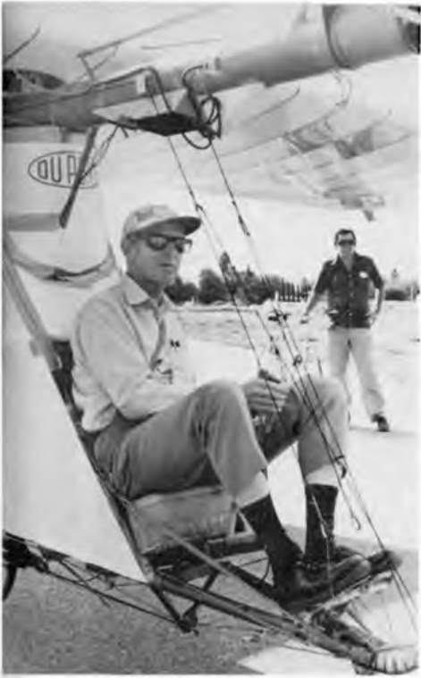
Left: Heath Robinson take note. Paul checks out the controls during the 'first test hop' even before aircraft was complete at Santa Susana. Streamlined fuselage fairing added later, allowing full access to all controls during this phase. Below: Janice-eye-view of cockpit layout, showing rudder, pedals and joystick, with instruments held in place temporarily with adhesive tape during early flights.
