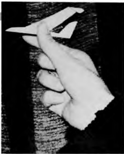
Left launching a paper glider to check the centre of gravity (CG) position Right a lot can be learned from making these small paper gliders
