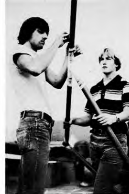
Left hand glider flyer Carlos Miralles (left) and model flyer Bobby Curtin, assemble fuselage frame tubes. Junctions are well reinforced with extra Kevlar cloth and epoxy. Below Blaine Rawdon, member of Cross-Channal Albatross crew, was responsible for most of the structural design on Solar Challenger, seen here on the tube wrapping machine strapping with Tedlar.
