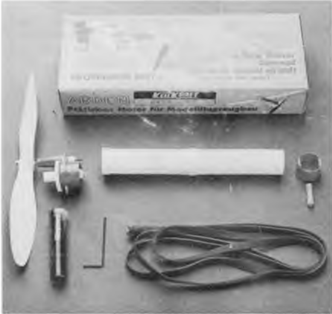
The component parts of the new Arden rubber drive unit distributed by Keil Kraft. The propeller is 175mm (7in) diameter. Photo A Callaghan
