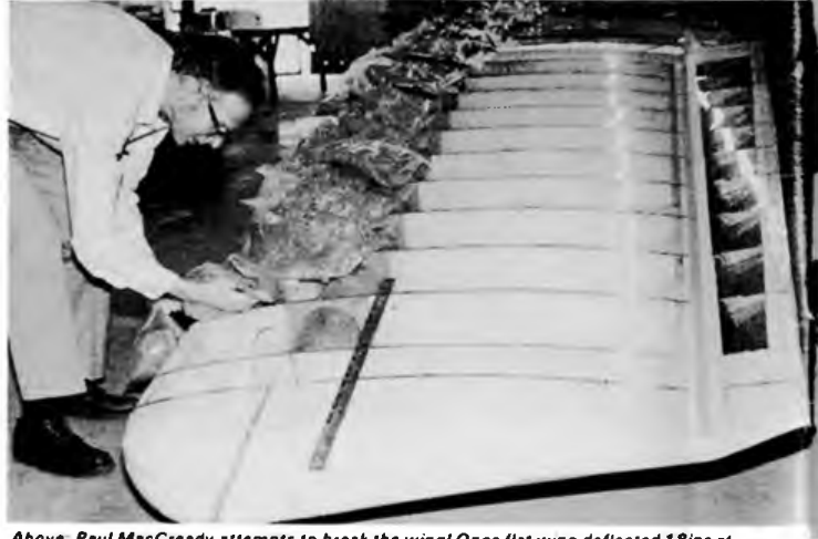
Above: Paul MacCreedy attempts to break the wing! Once flat wing deflected 18ins at tips to support almost half a ton of sand during positive +6G test. Unique flat topped aerofoil allowed upside-down construction. Below: here 1/4 in. expanded polystyrene wing ribs are threaded onto main wing spar.
