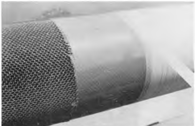
Outer wrap of Kevlar cloth being strapped in place with stretchy Tedlar tape while two part epoxy resin cures
