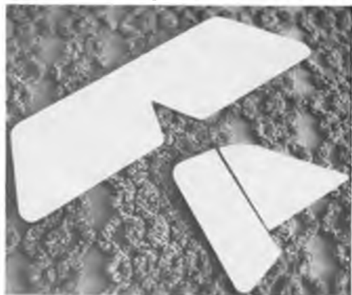
Left: the tailplane and fin as supplied with the kit. This could be improved by laying thin strips of balsa to the surface to represent ribs and spars, and then covering with tissue.
