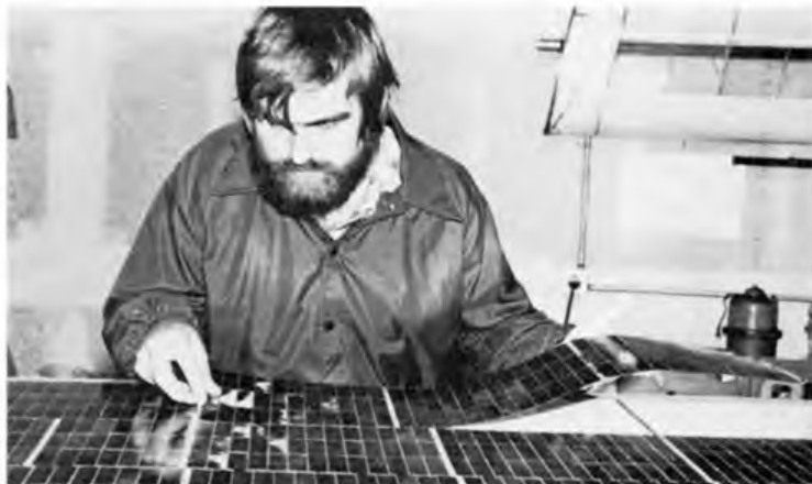
Ray Morgan adds another string of photovoltaic cells. A total of 16,128 cells covered flat top surfaces of wing and tail
