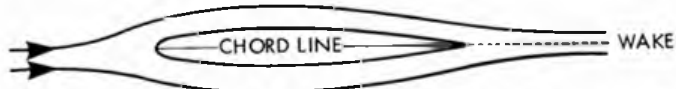
(b) Moderate angle of attack (Note curvature of flow upwash and downwash).
