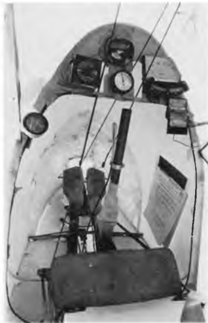
Left: Heath Robinson take note. Paul checks out the controls during the 'first test hop' even before aircraft was complete at Santa Susana. Streamlined fuselage fairing added later, allowing full access to all controls during this phase. Below: Janice-eye-view of cockpit layout, showing rudder, pedals and joystick, with instruments held in place temporarily with adhesive tape during early flights.
