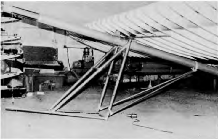
Above: bare bones of fuselage, test fitted to tail boom and wing, early during construction. All carbon fibre tubes around pilot were encased in Kevlar to produce safer failure mode. Below: 1/8 thou. inch heat shrink Mylar covering draped over underside of centre section by Ray Morgan, Steve Miller and Blaine Rawdon during covering
