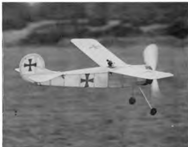
Coming in for a perfect landing after a good 30 second flight. Although the motor can take over 100 winds of the key, we found 90 turns gives very good flights and also prolongs the life of the rubber.
