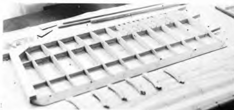
Left: structural modification made to the tailplane of the SE5A to enhance the scale appearance. Right: the wing under construction, note the riblets that were added to increase the scale effect of the wing.
