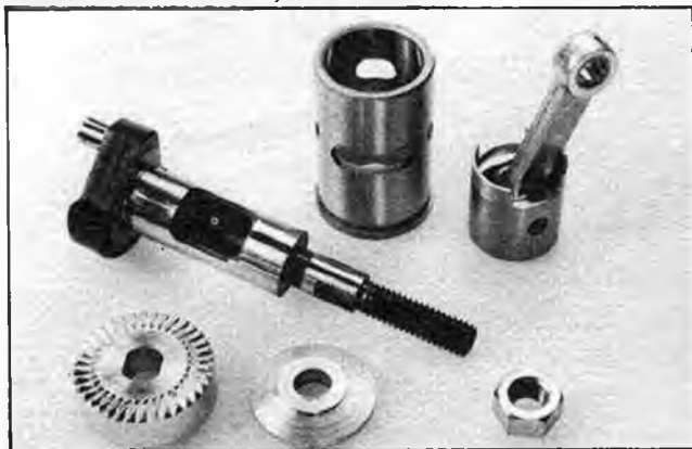
Crankshaft is orthodox; cylinder liner, of chromed aluminium alloy, is not. Note; hefty forged conrod.
