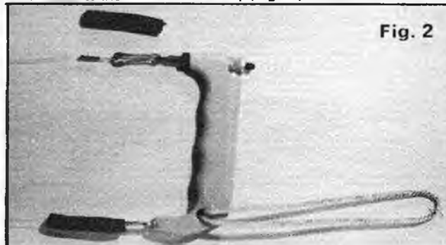
Fig. 2 Control line handle fitted with a strong wrist strap. Note the rubber tubing used to clean up line connections and avoid tangles with opponent's lines.
