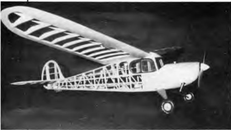
Above the Stentorian assembled, note the 'Bailey-Bridge' type of fuselage construction and the fact that the undercarriage legs are much shorter than those of the original model (see text) Right Phil Smith of Bournemouth patiently waits his turn to fly in the 1947 Bowden Trophy with his beautiful yellow and black prototype 'Stentorian'
