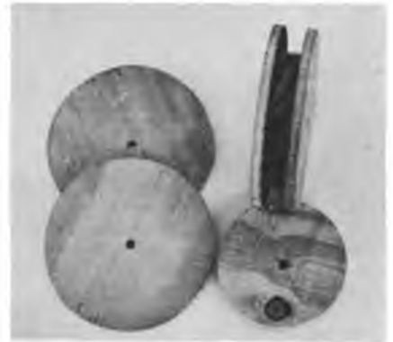
The central line storage reel is simply made up from two large diameter plywood discs and a more substantial thickness centre spacer. Centre drill the discs and be sure that the joint is sealed so that the wire cannot be trapped between the discs.
