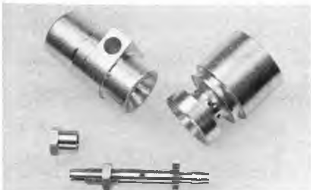
Special intake venturis for Super Tigre. Small one is for X15 Combat engine. Larger one is for conversion of ST60 to C-1 stunt use.
