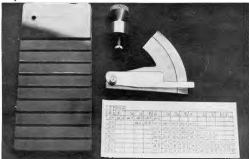
Above left: the prop balancer baseboard made up from layers of perspex. Note the hole top left for the prop carrier. Top centre — the prop carrier made up in part from a Micro-Mold propeller balancer. Modified protractor with cursor in place is in centre of picture above the pitch read-off chart.
