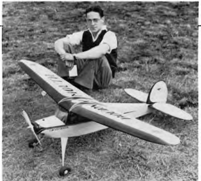
Above the Stentorian assembled, note the 'Bailey-Bridge' type of fuselage construction and the fact that the undercarriage legs are much shorter than those of the original model (see text) Right Phil Smith of Bournemouth patiently waits his turn to fly in the 1947 Bowden Trophy with his beautiful yellow and black prototype 'Stentorian'
