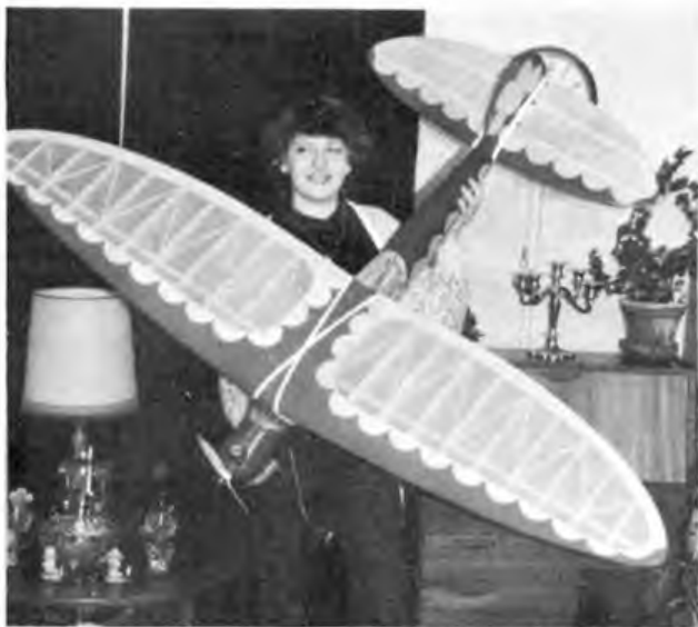
Left double sized Keil Kraft Kits 'Scorpion' by Peter Elmer of Cardiff shows well the spars, wide rib spacing and diagonal rib bracing in the wing structure. Above Ken Hinton's 'Answer' no spars in that 'Ritz-Wing', but ribs are spaced only 1in apart over the completed wing panels. The 'Answer' was kitted in USA as the 'Bay Ridge Topper' in 1940.
