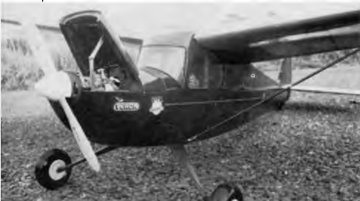
Below close up of nose showing the engine room hatch in the open position over the ETA 29 glowplug engine and the attractive original transfers (see text)
