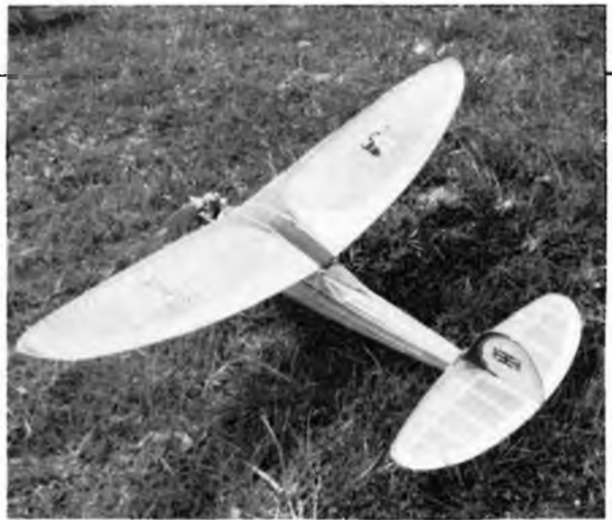
Left double sized Keil Kraft Kits 'Scorpion' by Peter Elmer of Cardiff shows well the spars, wide rib spacing and diagonal rib bracing in the wing structure. Above Ken Hinton's 'Answer' no spars in that 'Ritz-Wing', but ribs are spaced only 1in apart over the completed wing panels. The 'Answer' was kitted in USA as the 'Bay Ridge Topper' in 1940.
