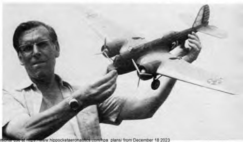
Right: another twin rubber-powered flying scale model. Derek Camps with his Martin B-10. 35in. span machine made in 1939 from an Ideal kit. The two apertures on the top wing surfaces aft of the engine nacelles are for the motor sticks, necessary to provide length of rubber when the model is used in the flying scale category.
