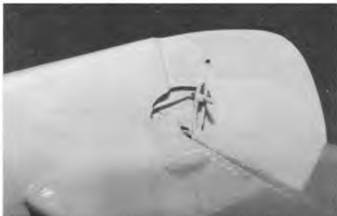
Control linkage detail. Above: view showing elevator push-rod and sideways location in slotted former also illustrates rear wing mounting. Right: elevator horn with adjustable soldered brass pushrod bush.
