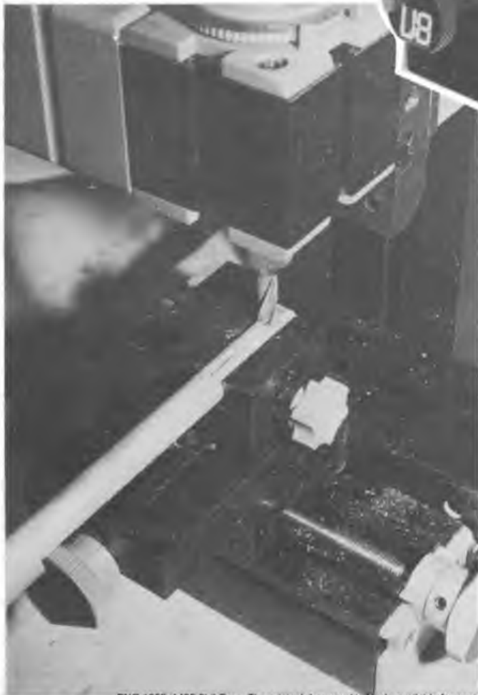
Above: the Unimat 1 in its most basic and probably most used format, the lathe. Left: vertical milling is just one of the many possible alternatives available.
