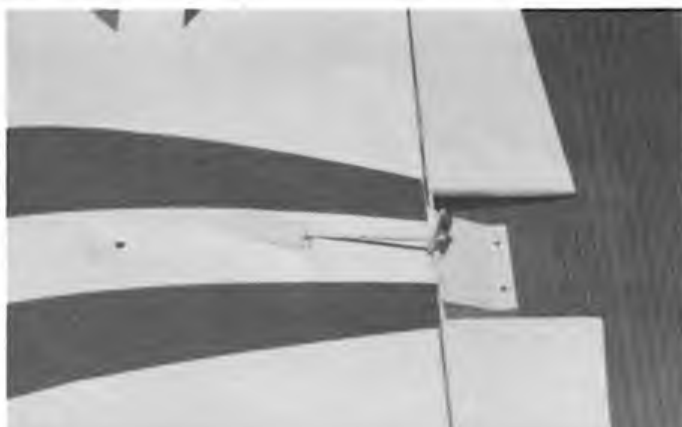
Above: tank and hatch cover fittings, tank is retained by single bicycle spoke across the fuselage and through brass tube soldered to tank. Note wing mount bolt and large nylon washer. Right: flap control linkage on upper surface of wing.
