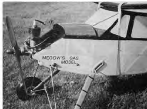
Below: Pat Fillingham, retired after a lifetime of test flying has exchanged his full-size 'Mosquito' for this 10cc OK 60 ignition powered example of Megow's 'Flying Quaker.' In this close-up note the varnished and bound undercarriage legs and that rivetted aluminium to cowling!
