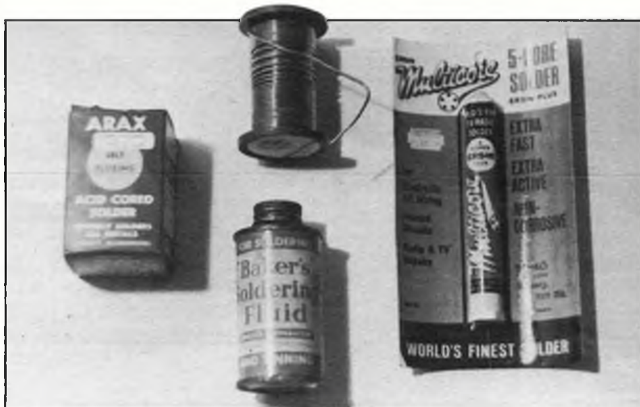
Above: various solders are available, left, an acid cored solder for piano wire, centre solid (non-flux cored) solder with Baker's Fluid flux and right, resin cored solder - the most widely available which is as near as possible to Tinnans solder.
