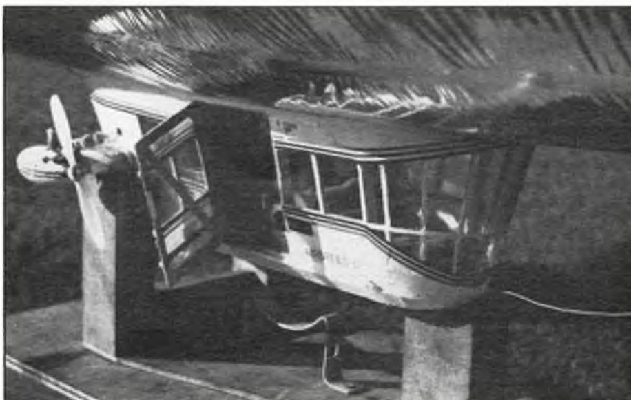
With model airships, weight could well be critical - there is only room for so much gas in the bag - so while some internal detail is provided in the gondola...weight precludes too much detail...
