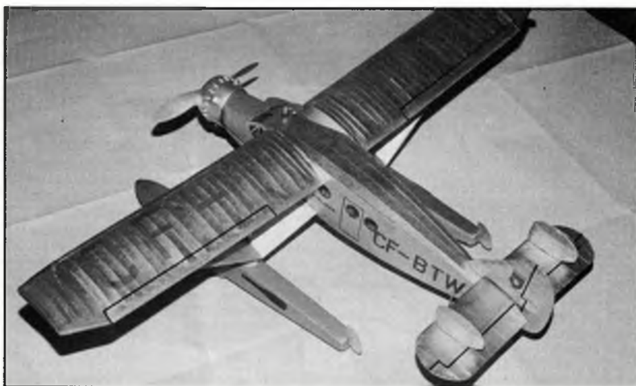
Two views of Barry Hetherington's Bellanca Aircruiser floatplane; 22in span and Telco powered. Note the scale structure; model weighs approx 60 grams but flies well. Characterful aircraft must be an interesting sight when airborne.
