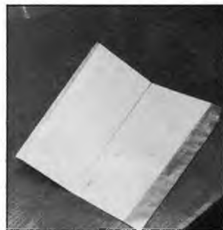
Small-scale sample of foil and balsa laminate arranged as it would be for wing construction. Note gap to allow fold and leading edge carbon reinforcement.
