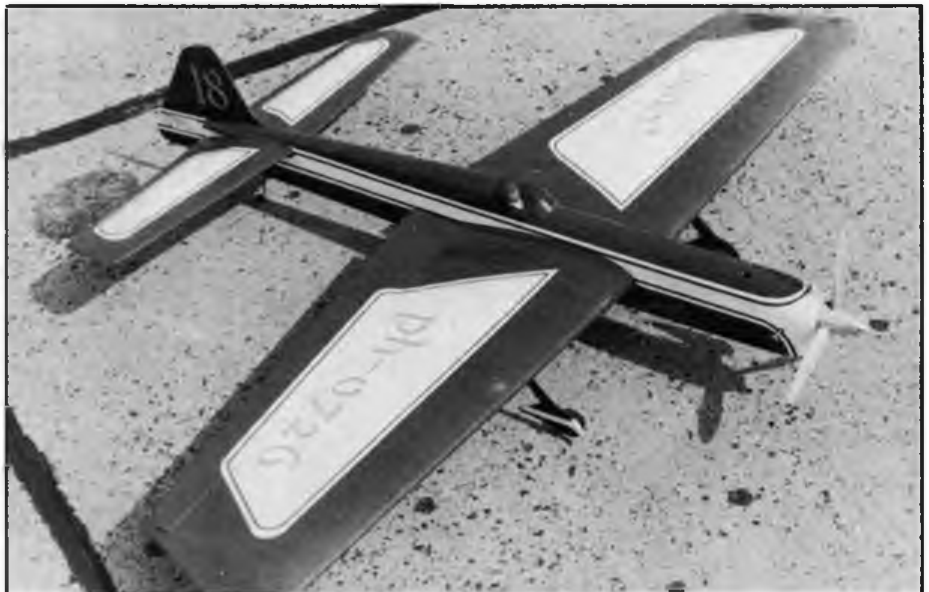
Top: How modified designs evolve - first obtain your plan! Above: Henk de Jong's elegant Juno Plus, S.T. G21/46 powered. Sleek model is finished with two-part acrylic car paint. Constructional differences between this and the original Juno detailed in text.
