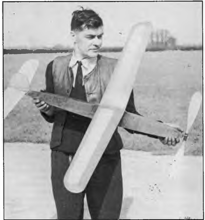
Eric Smith with his Themis Wakefield, designed to be the ultimate, and described in Aeromodeller. Notice feathering prop, tip-tail D/T and beautifully faired wing mounting.
