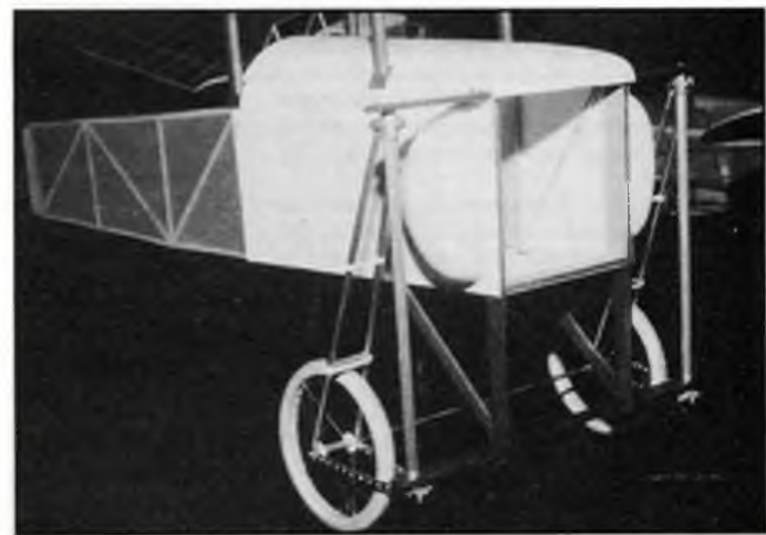
The fully sprung undercarriage and vacuum-formed panelling of Paul's as yet unfinished 'large' Bleriot. Attention to detail is remarkable.
