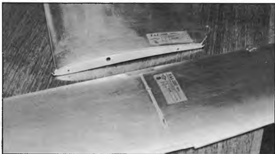
Stafford Screen's most recent covering effort - immaculate. Root of wing shown at top; below is tailplane on which leading edge recess for mounting and pivot are clearly visible. Hooks at wing LE and TE allow halves to be bound onto fuselage with rubber bands. Two-piece wings are a new departure for Stafford.
