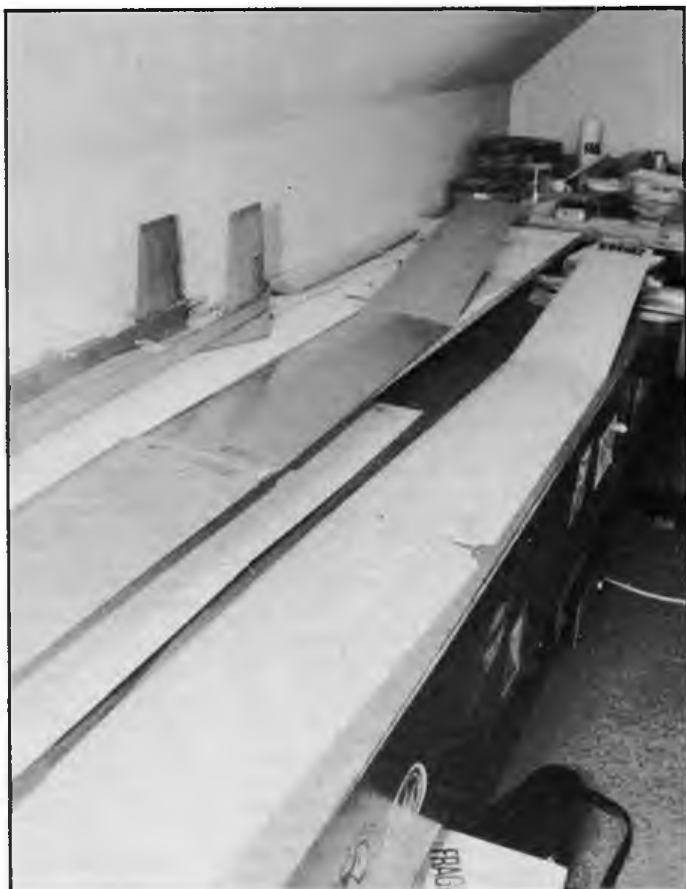
A part of the workshop showing finished foil-covered wings with an identical balsa pair. The idea is to rough-trim the model with balsa wings and replace by foil wings for last trim flights and contests.
