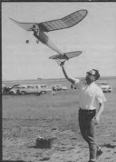
Above: One of the most shapely C E Bowden designs, this Mills 1.3 powered 48in span Satellite was made by Paul Lidster and is seen at the 1987 Vintage Weekend. Plans available from Phil Smith.
