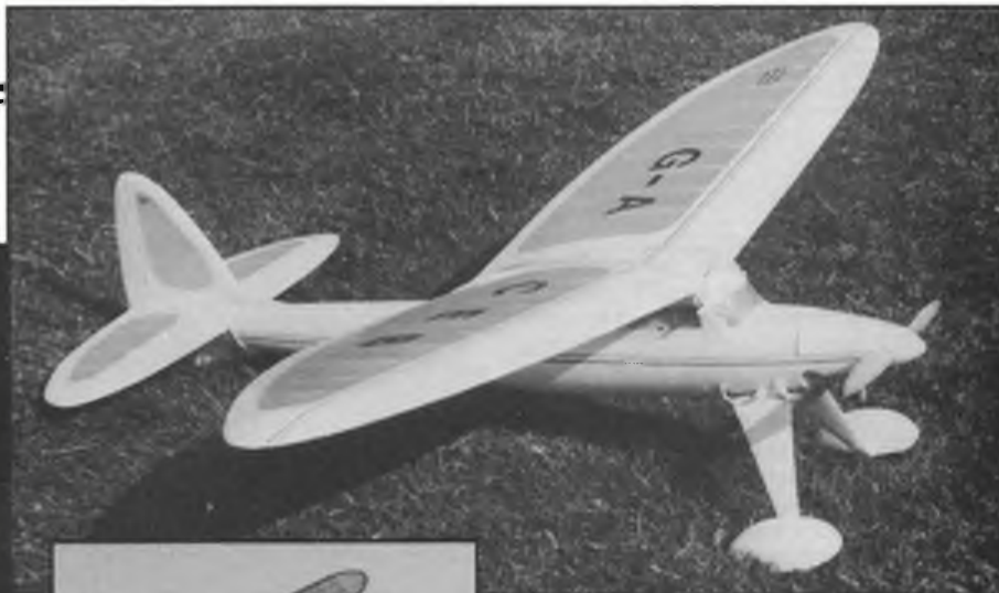
Above: One of the most shapely C E Bowden designs, this Mills 1.3 powered 48in span Satellite was made by Paul Lidster and is seen at the 1987 Vintage Weekend. Plans available from Phil Smith.
