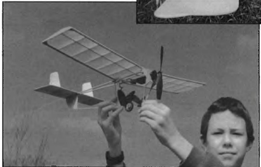
Top: Peter Lang's own-design, all-sheet sports soarer is 48in span. Union Turbo MO-7 motor/gearbox; six 600mAh cells. Above: Our columnist's 'Demoiselle-style' microlight for K&P O1 power. Right: Couldn't be much simpler, could it...
