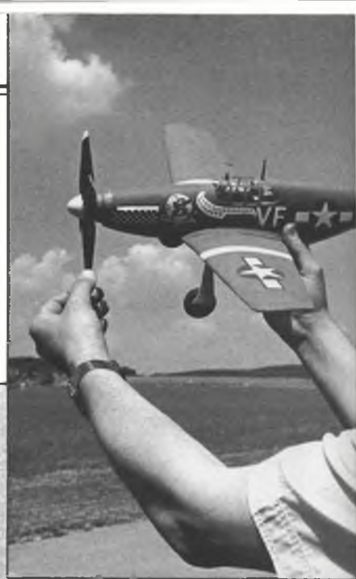
Above: Zdenek Poduska's P-51B is his first model! All-foam construction means it's relatively heavy at 65gm but model flies stably for up to 45 sec. All photos this page: Ivo Ceresnak.
