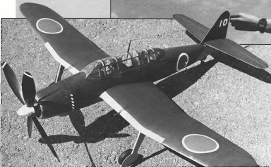
Left: Another subject by Vladimir Kunert (senior!), this Aichi A6M Grace spans 720mm and weighs 110gm with 25gm motor. Flights in excess of 110 seconds are regularly achieved, which accounts for the incorporation of a parachute D/T (actually hidden in the ventral radiator). The majority of rubber scale models in Czechoslovakia are built to 1/20 scale; prop diameter is limited to 35 per cent of span.
