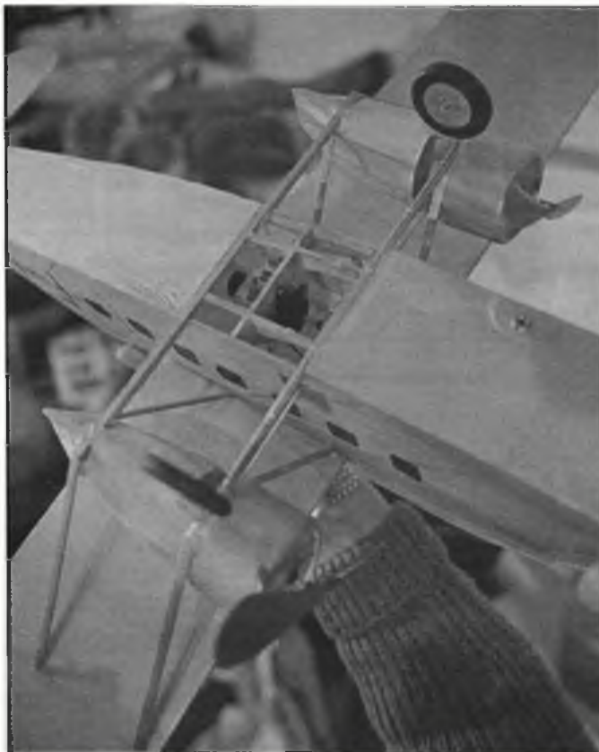
Derek Hardman's large Potez Indoor scale craft features single K&P motor with flexi-drive to twin props. Hmmm...
