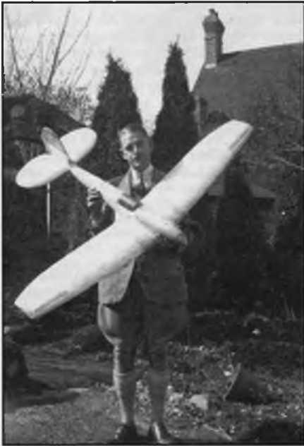
Doctor Forster in April 1942 with P-10, his experimental low-wing model, a semi-scale Spitfire, that was used to evaluate several features that would be used on a near-scale Spitfire. Note wing-tip slots and clipped wings, the latter to receive lightly glued-on, knock-off tips.
