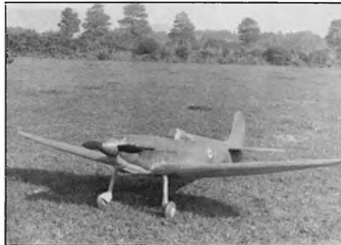
P-11 was a flying scale model of the Spitfire II powered by a buried 6cc Baby Cyclone. Plans were available from Aeromodeller Plans Service, and despite Doctor Forster's warning that it was not an ab initio petrol model, some beginners at power model flying chose it as their first model! One wonders how they fared . . .
