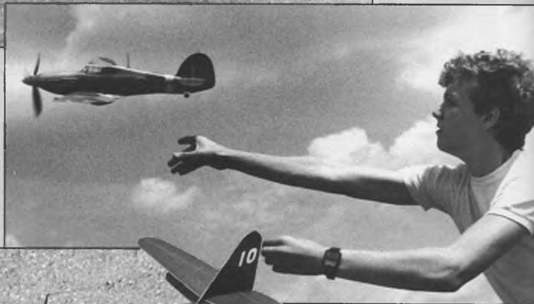
Left: Another subject by Vladimir Kunert (senior!), this Aichi A6M Grace spans 720mm and weighs 110gm with 25gm motor. Flights in excess of 110 seconds are regularly achieved, which accounts for the incorporation of a parachute D/T (actually hidden in the ventral radiator). The majority of rubber scale models in Czechoslovakia are built to 1/20 scale; prop diameter is limited to 35 per cent of span.
