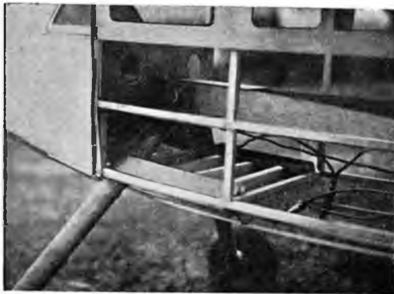
The time switch is located on a panel of three-ply fixed to the bottom longeron and the one above. In front of the switch is the connection for plugging in the "booster" accumulator.
