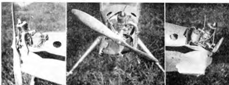
Three entirely untouched photos, showing the exact amount of "damage" sustained by the 100 ft. dive on to Fairey's Aerodrome, which is described in the article.
