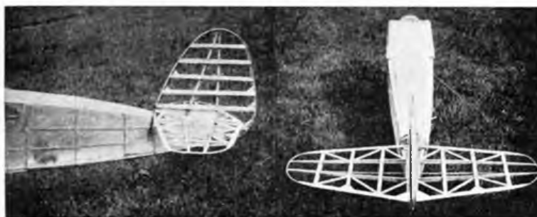
On left may be seen the rubber band suspension for the rear wheel, and on right views of the fin and stabiliser.
