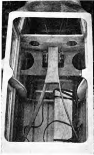
This photo shows one of the steel tube chassis legs projecting through the slot constructed in the bottom side of the fuselage.
