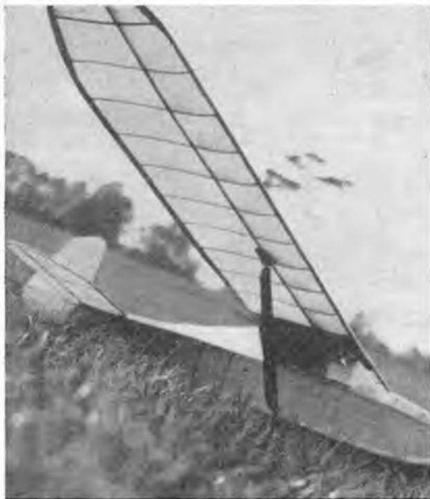
An interesting semi-scale model of a German intermediate sailplane. This machine, weight 8 ozs., span 50 ins., has obliged its builder R. Anthony with 5 mins. o.o.s.
