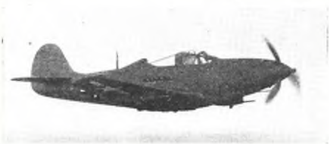
The latest version of the Bell P-39 Airacobra is armed with a 37 mm. cannon firing through the spinner, two .5 machine-guns in the motor cowl-ing and a 20 mm. cannon below each wing. (Photo: Bell Aircraft Corpn.)
