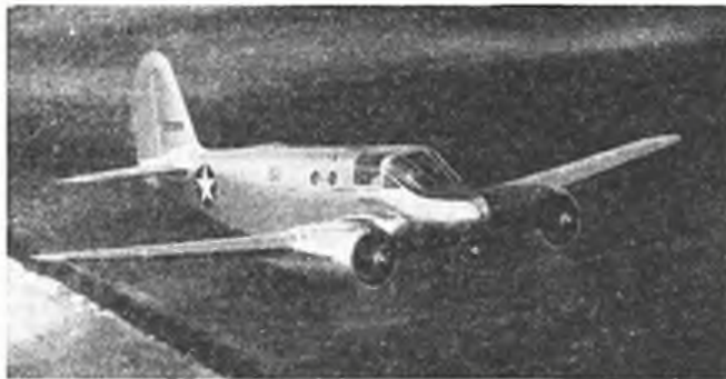
The Beech AT-10 Wichita transitional trainer. The motors are 275 h.p. Lycomings. (Beechcraft photo.)
