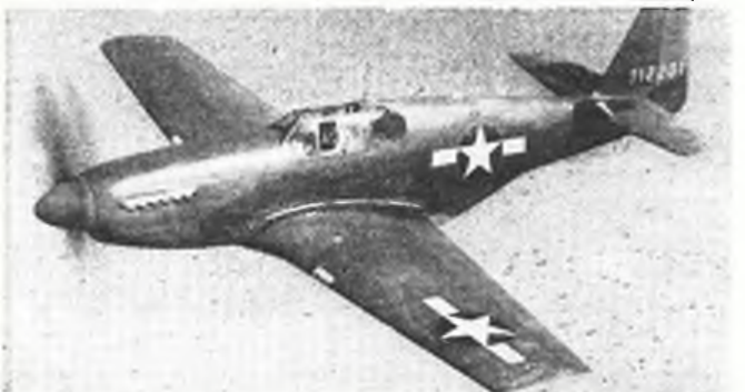
The P-51B Mustang with Packard-Merlin motor known in the R.A.F. as the Mustang III. (Photo: North American Aviation.)
