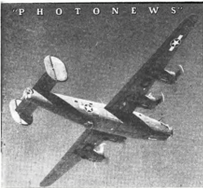
The Consolidated B-24J Liberator, with four 1,200 h.p. turbo-super-charged Pratt and Whitney Twin-Wasp motors. (Photo: Consolidated Vultee Aircraft Corpn.)
