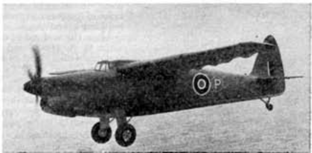
Pastures New. One of the two prototype Supermarine S.24/37 aircraft fitted with variable incidence wing. First built in 1943, these aircraft fulfilled a Naval torpedo-bomber requirement. (Vickers Photo.)
