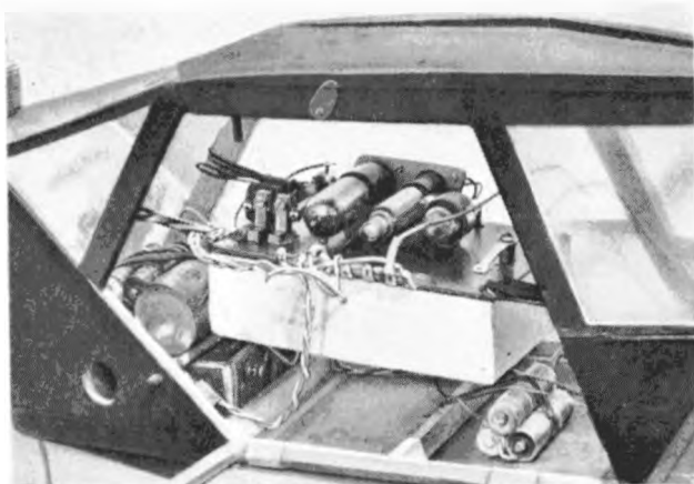
E.D. receiver installation. The protective base is left on to keep out dust, etc., and also saves a lot of damage in the event of a prang. Right, is G. Hannest-Redlich, designer of the E.D. equipment, shown here with his "Electron V" at Fairlop where he won the Ripmax contest.
