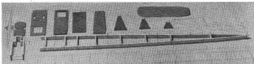
1. Crutch is first pinned down: formers can be cut while cement dries. Note that formers subject to stress extend through to bottom of crutch.
