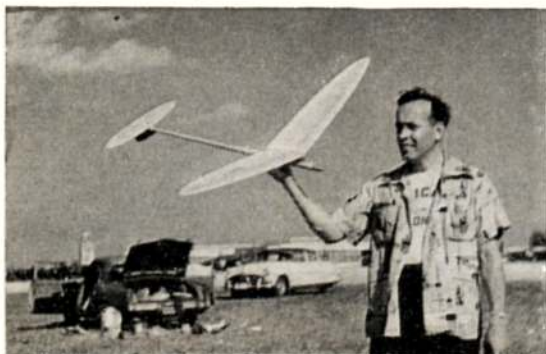
Above, Gerry Ritz of Chicago, U.S.A., with this beautiful A11 at the Miami International Contests, Florida. Model has typical Ritz wing with curved plate section, is sparless with elliptical outlines. At right is the line-up of stunt entries at SOUTH AFRICAN Nationals in Johannesburg at Easter
