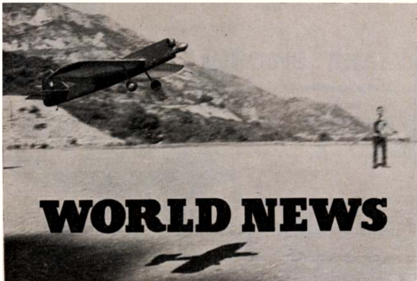
From Menton, FRANCE, R. Bardou sent us this action shot of his fibreglass stunt model. Weighing only 27-oz. for 50-in. span, fuselage is an elliptical section tube, wings have balsa ribs set into fibreglass moulded leading edge
