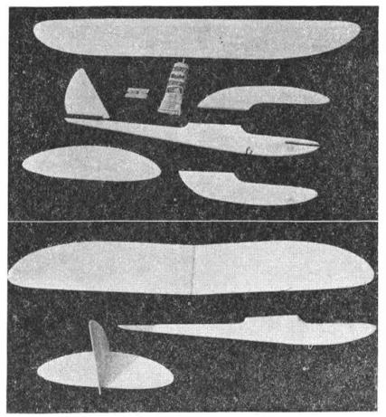
Component parts of WHIZLER at left emphasise the simplicity of Keith Laumer's speciallycreated design to launch this new series for the novice arromodeller. Fuselage side doublers add considerable strength and leave an open slot in the nose for trimming weight to be enclosed, and finally blocked in with a piece of baiss. Razor blade, cement and sandpaper are the only accessories one needs to make this fine 24-Inch span flyer
