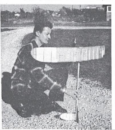
motor at 0 deg., drag is quite low; in addition, these design features provide excellent transition from the "straight up" climb to glide without tricky mechanical means of changing incidence. The low wing is positioned for a good glide, as the tailplane is out of its downwash.
