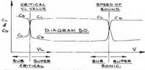
The approach to the smaller model is to use sections of low critical VL which will be exceeded in normal operation. To enable some of the methods of obtaining a low critical VL we must first understand what causes the critical VL effect. When air flows past an airfoil section, there is a very thin layer next
