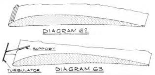
without them; also Lindner in 1954 and 1955 used one of Hacklinger's sections without a turbulator and with no ill-effects. Many results obtained in wind tunnels are fictitious as a low speed wind tunnel is quite likely to be turbulent.
