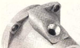
★ Air-intake venturi on underside of front housing.
