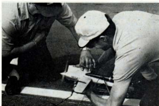
Jack Frye hand starts his .65 powered model while Jerry Roselle holds. Hand starting is used to avoid loading the bearings on this precisely set-up motor.
