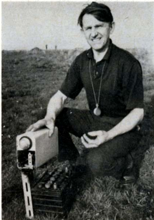
Left, K. Attiwell with his own designed towline pull tester - constructed from Dexion, Meccano, a spring balance, micro switch and an indicator lamp from an Austin A.30. The unit can be adjusted for calibration with standard 2 kilogram weights. When a 2 kilogram pull is applied the light comes on, and could be very useful as a standard towline tester for all Area and National events, etc. A 12v. car battery is used to stabilise the unit.
