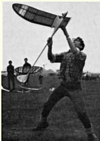
Andrew Brewster prepares to launch his Rossi 15-powered F.A.I. model. Very fast, even at testing stage, engine performance indicating that the days of the Super Tigre G.15 being the automatic choice, are numbered.
