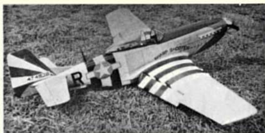
Ken Whenham's winning control-line scale Mustang is 46 in. span and weighs 5 lb., powered by a Merco 35. Heavy landing during a qualifying flight knocked several pieces off, but did no structural damage.
