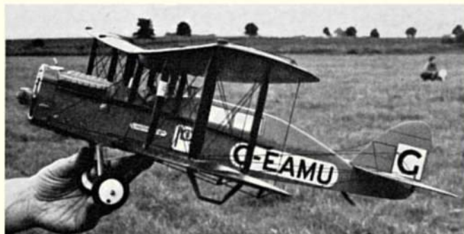
Ken McDonough's D-C Dart diesel-powered Instone Airlines D.H.4a weighs only 8 oz. fully rigged and ready for free flight.
