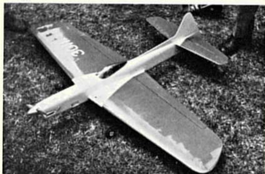
Paul Turner's winning stunt model has Fox 35, and is his own design. It has no development history, being the first of a future series, in which the first mod will be to make the wing asymmetrical.
