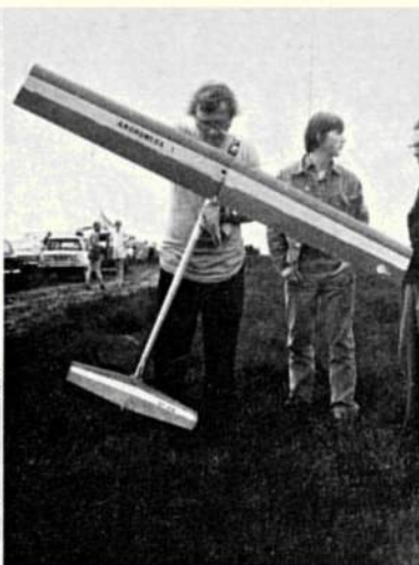
Danmark's Thomas Koster with his all-wood model. Four-function Seelig timer operates motor, auto-rudder, then variable camber wing and V.I.T. simultaneously, and finally D/T. Wings are one piece and bolt on.
