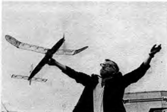
John O'Donnell launches his Nats fly-off, 400 ASA film 1/1000 sec. shutter speed. Wing appears kinked due to an illusion created by partial masking by propeller.
