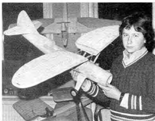
Dornier Project Do-245 with monocoque fuselage weighs 70g and is reported to fly very fast. Right: George Worley holding his father's own design Douglas O-46A destined for Icc diesel power. 1:12 scale model is 45in. span and weighs 20oz as shown.
