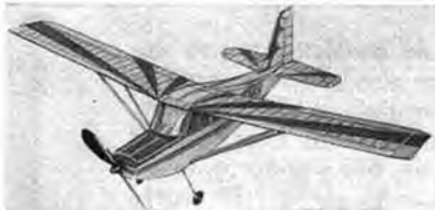
CITABRIA 23" (584mm) Span. One of three Pre-decorated, All-Diecut Scale Flyers, Rubber driven. Others are Skywagon and Bolkow Junior. Ideal for Telco CO 2 motors. Kit Price £2.35
