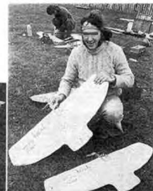
Below: The Tribe brothers flew this model with retractable undercarriage and single blade prop. Dave Willis with his Rossi powered Boomerang models, glass cloth centre covering made them really tough, used vac-formed pacifier pods soon to be commercially available.
