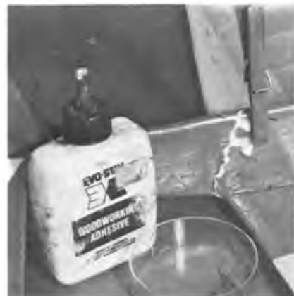
Below: Long jagged breaks provide plenty of surface area for gluing parts back together. Right: Hold with pins, pegs, tape, etc. until dry, but make sure parts are aligned correctly.
