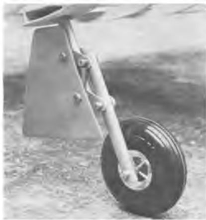
Opposite: Brian Dyke nearing completion of his latest monster stunter, this time a Westland Wyvern - what a craftsman! This page: Close ups confirm the quality of work and attention to detail, note parallelogram sprung shock absorbers on undercarriage leg left.
