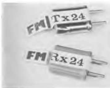
Above: another complication – FM means Frequency Modulation rather than 'failed miserably' and denotes a new type of R/C system now becoming more generally available. Crystals without the "FM" notation are "AM" or amplitude modulation type. Basically, the two types are incompatible so don't put AM crystals in FM R/C sets and wicky works!
