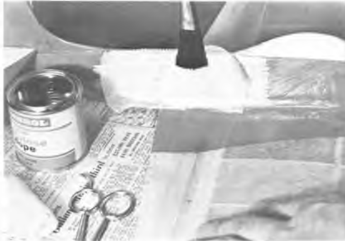
Left: Most glue joints will prove stronger than the original wood, but extra reinforcing can be added by covering with bandage patch applied with balsa cement or dops.
