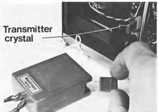
Below: R/C manufacturers go to lengths to ensure transmitter and receiver crystals are not transposed. In MacGregor set, receiver crystal fits into plastic key, which slots into receiver – foolproof! Picture right shows how. Set supplied for photography by Waller & Arris, Hemel Hempstead.
