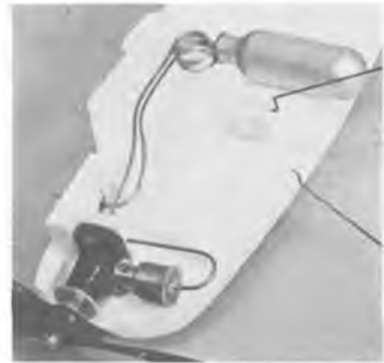
Far Left: Here's Telco, and this is what you get in the box; model comprises of simply five major components which quickly assemble into a first class flying model. Left: Plastic mounts for motor, filler and undercarriage slot into expanded foam fuselage halves. Above: Fuselage halves joined shows patch of Scotch Tape on wing platform. Button of plastic protrudes to accurately locate wing.
