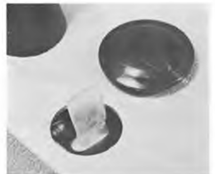
Below: plug-in crystals for R/C systems are the norm. On Skyleader transmitter, crystal slots into holder under case top and is protected by plastic cap.
