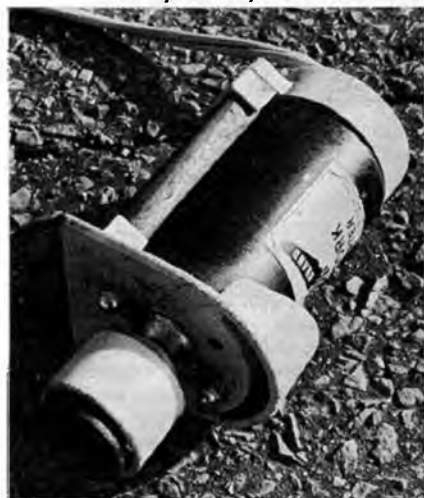
Below: A handy gadget for any R/C power flyer with sore fingers, this Sullivan Pylon Brand Hi-Tork electric starter is powered by a 6 volt accumulator.
