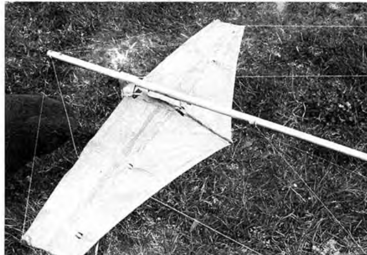
Above: Slot lip ailerons, as tried on Toucan MPA, proved the solution to lateral control. Holes in surface allow some air through even with flap down, thereby reducing unwanted tip stalling.
