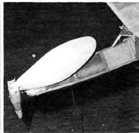
Folding propellers, as on this Mercury Mentor reduce drag improving glide.
