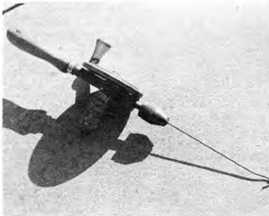
Hand drill fitted with wire hook for winding rubber motor.
