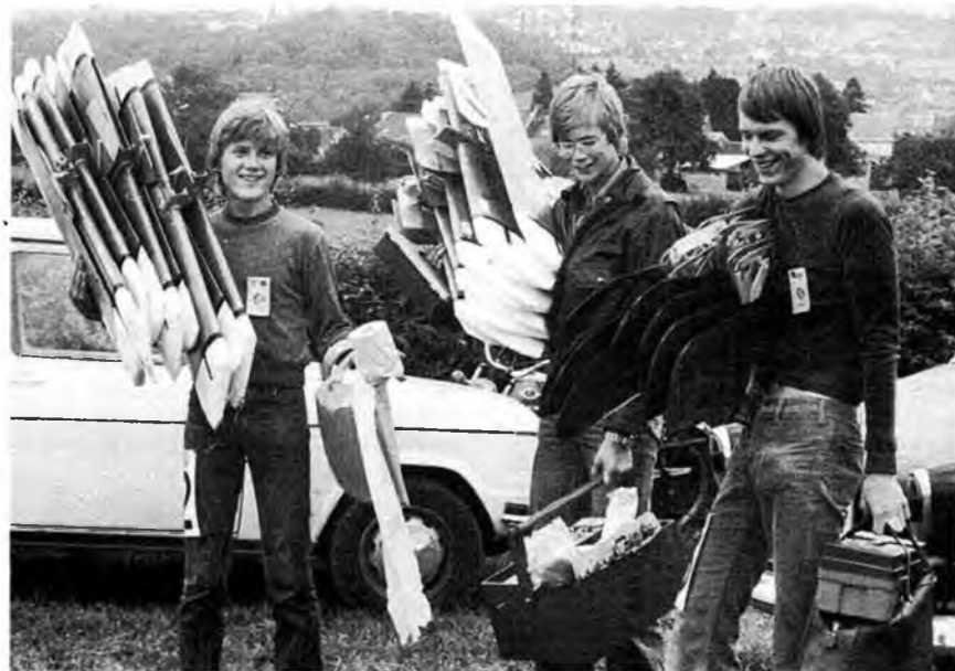
Current FAI rules encourage lightweight disposable models. Flyers frequently require 6-10 models per contest! Pictured here are Swedish combaters Per Stjarnesund, Johan Norelius and Johan Sandstrom with the armfuls of models they used at Verviers, predominantly mass produced foam polystyrene construction powered by Rossi 15 motors.
