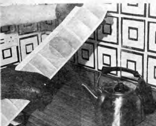
Twist the wings over a steaming kettle to achieve the correct warps.
