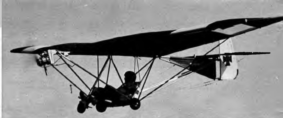
Another new shape in the skies; powered micro-light aircraft which use hang glider technology fabric wings, combined with spartan accommodation for pilot. Above: John Chotia's Weedhopper from Utah, USA. Right: Steve Hunt, Chairman of newly formed BMAA at the controls of his Hiway Skytrike which uses add-on hang glider power unit.
