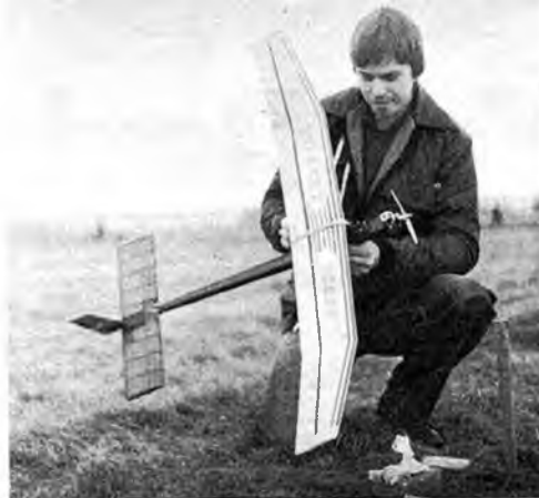
Above: Frank Rushby of Grimsby club flew this 1A model with 9% thick wing sheeted top and bottom; TD .049 swings Tornado 5 1/2 x 3 prop. Model now weighs 8 1/2oz.
