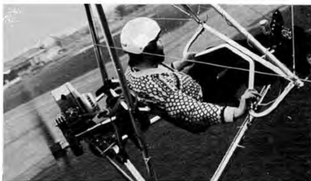
Another new shape in the skies; powered micro-light aircraft which use hang glider technology fabric wings, combined with spartan accommodation for pilot. Above: John Chotia's Weedhopper from Utah, USA. Right: Steve Hunt, Chairman of newly formed BMAA at the controls of his Hiway Skytrike which uses add-on hang glider power unit.
