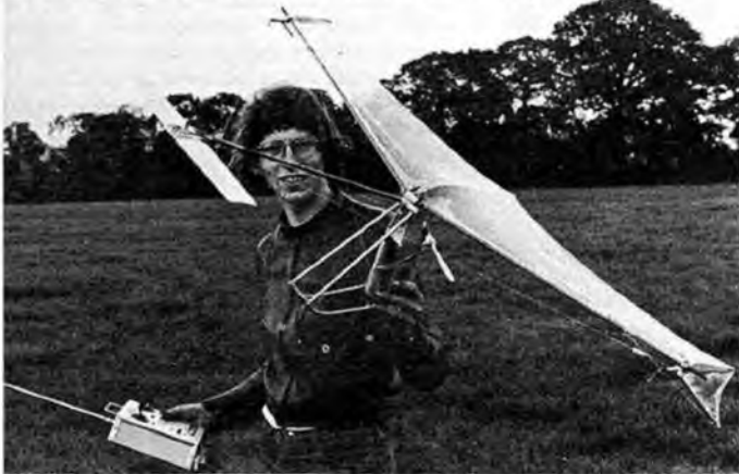
Below: Original 1200mm span 2 channel R/C model powered by .8cc Cox Baby Bee. Note plastic covering film pulled taut over centre keel rib, and 'Cyclone' type droop tip fins.
