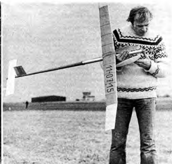
Visitor at Midland Area Gala from Germany was Lothar Döring with this all sheet F1B Wakefield. Black chord wise stripes on wing are carbon fibre reinforcement stiffeners. Top left: Wind and air temperature pen chart recorder, used to help detect passing thermals. Below right: Modified Seelig timer uses wire latch to control timer start, arms are hinged in dural plate. Below left: Plug on tips are accurately located at trailing edge with neat brass wire clips allowing wash-out adjustment.
