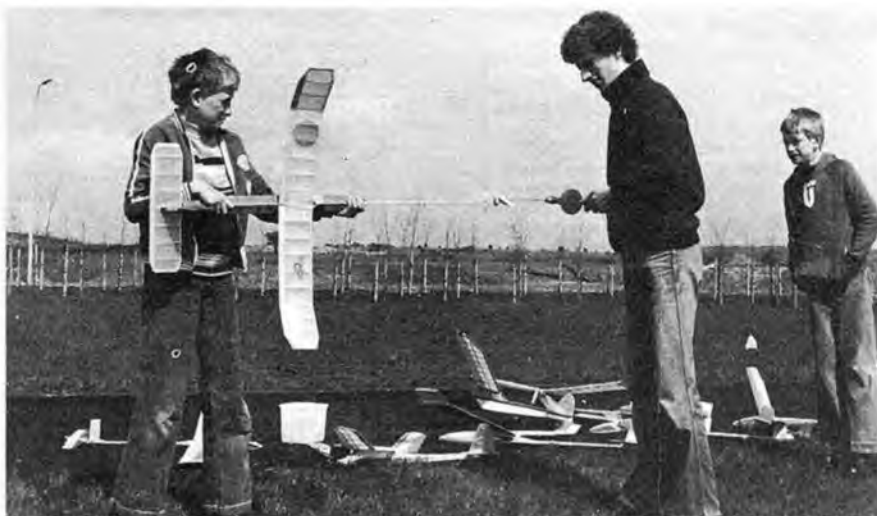
Rubber motors should be stretch wound, with assistant taking all the load only on the rear motor peg.
