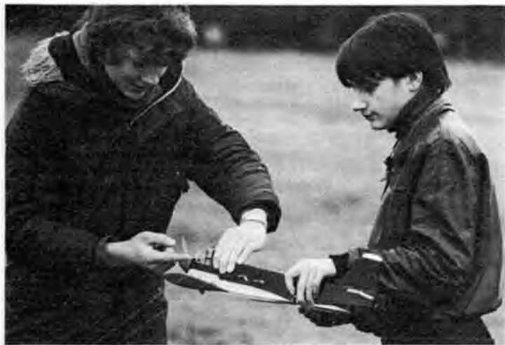
When starting the engine it is advisable to get your assistant to hold the model steady and grip the fuselage around the engine for extra support.
