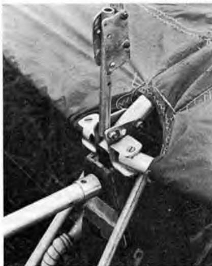
Above: Simplified underslung pod made from alloy tube for R/C equipment and Mills .75 motor. Below: Kingpost incorporating 'over-centre' hinging break to release tension in wires for adjustment or derigging on 10cc version.
