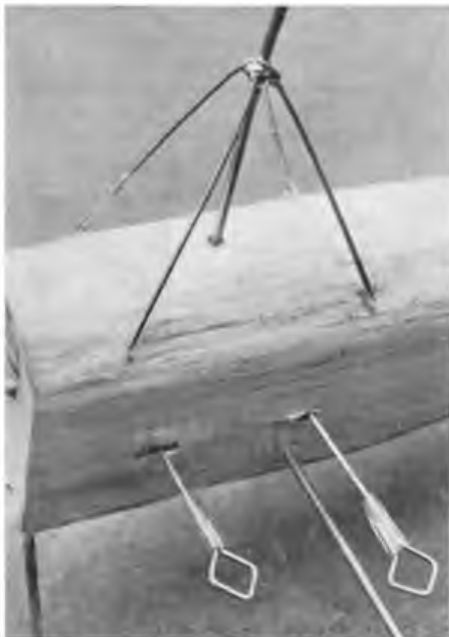
Right: sew and epoxy the pylon wire to the appropriate former.
