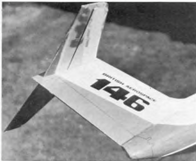
Tail assembly showing the 146 logo and fine line markings to indicate rudder hinge point.
