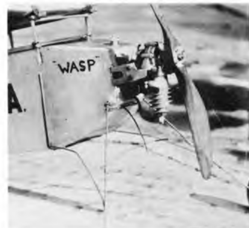
Below: close-up of the Elf engine showing the "full-size" propeller hub, and the pleasing shape of the Chauviere wooden propeller. The "main" fuel tank was made of sheet brass and was mounted in the front fuselage bay supplying the jet via a float chamber. Note the toothpaste tube filler cap!
