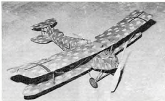
Left: Mike Hall's 1:24 scale version of the Hannover CLIIIA was powered by a Telco motor and flew well. A great deal of work is involved in that colour scheme together with the scale details.
