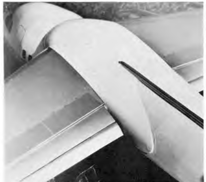
Right, detail of the wing fairing. Left shows the KeilKraft 4552X motor installed in the inboard nacelle. Propellers used were 4" diameter as supplied by KeilKraft. Note the mock-up fan in the outboard engine nacelle.
