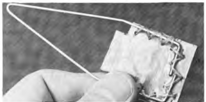
Below: balsa fairings are epoxy glued to the wire rotor pylon, and top surface of the surface
