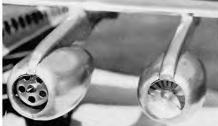
Right, detail of the wing fairing. Left shows the KeilKraft 4552X motor installed in the inboard nacelle. Propellers used were 4" diameter as supplied by KeilKraft. Note the mock-up fan in the outboard engine nacelle.
