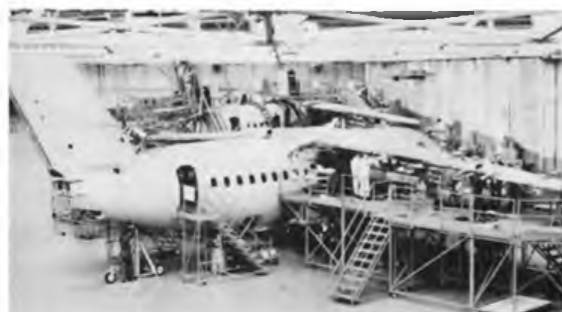
Prototype BAe 146 in final stages of assembly just a few months prior to roll-out. Below: for modellers a detail of the wing with Fowler-type flaps extended.
