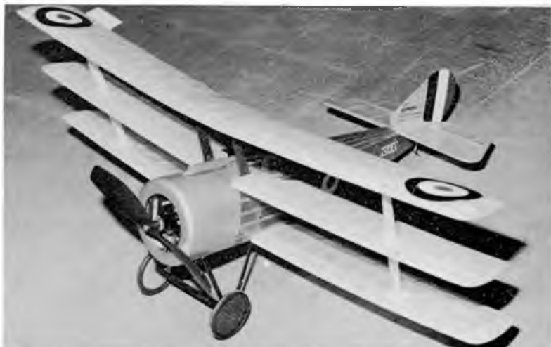
This CO 2 conversion of the Veron Sopwith Triplane flew very steadily for its builder Pete Iliffe. Simply finished in tissues, it was very neatly built.
