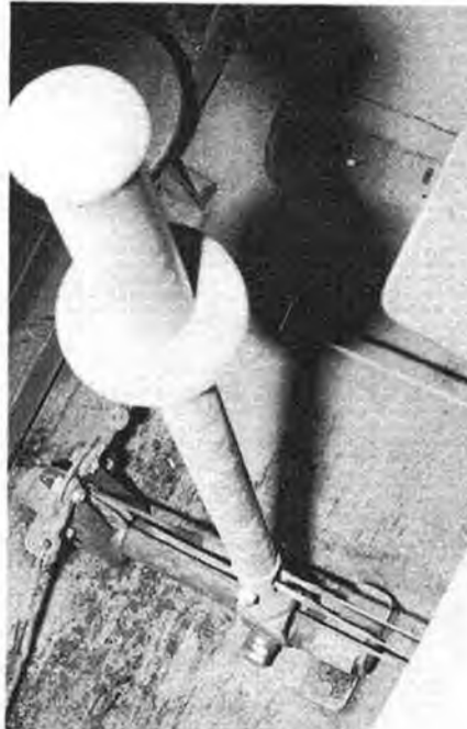
Close-up of control stick, cables and pulleys on cockpit floor.
