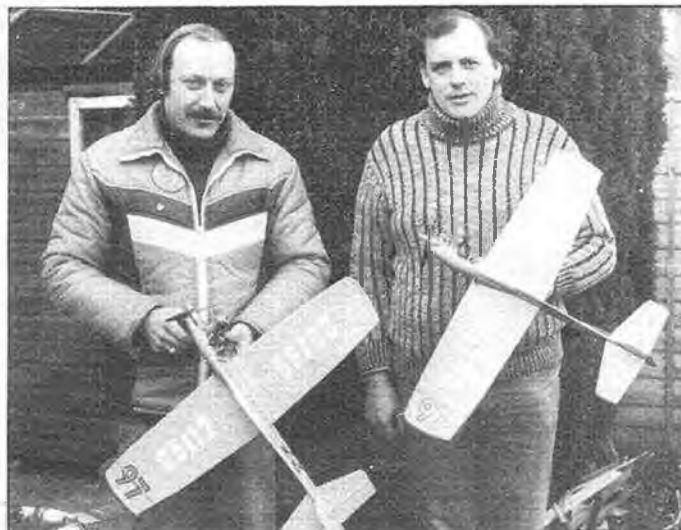
Above: Catlow-Jephcott model, APS OL' Blue design, Nelson 15 G/D 2.5 engine. Note: filler/shut-off between tank and engine. Few teams use regulation spinner nut as shown here, despite being demanded by the rules.
