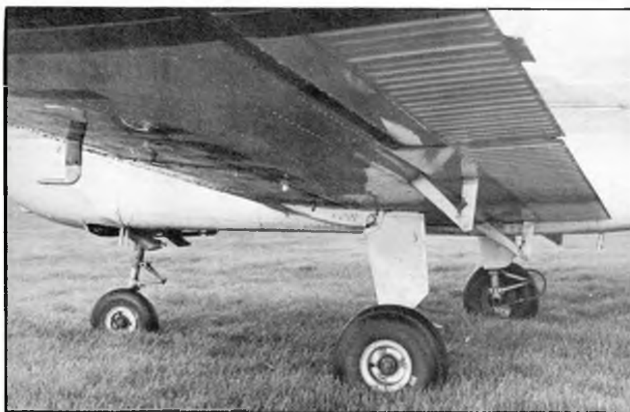
Top: shades for the 'breakfast patrol' - Fuji 200 slips in low past the trees! Above: wing underside detail showing the main undercarriage, and the flap hinge line. Above right: the Fuji 200 tail cone - note the 'inverted' horizontal tailplane airfoil section distinctly visible. Right: for those thinking in terms of the ultimate in scale modelling detail, here is the Fuji 200 cockpit instrument panel.
