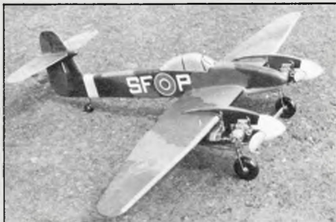
Some interesting examples of profile scale designs. Top left: Westland Whirlwind twin by Derek Bird of Three Kings Club for two P.A.W. 149 motors. All sheet, but non-aerobatic. 2nd left: twin Grumman Tigercat is capable of aerobatics. 3rd left: Japanese Kawanishi by Bernard Sexton of Three Kings uses 3-line control. Aerobatic on O.S. 19 R/C. Below: really original - Macchi MC72 by Geoff Burkett uses 3-line control. P.A.W. 19 power. Floats have piano wire runners for take-off, sparks and all! 2nd right: Heinkel UHU twin from Broadlands Club, Norwich, fully aerobatic on two 35 motors. Bottom right: the author's Hawker Hurricane.
