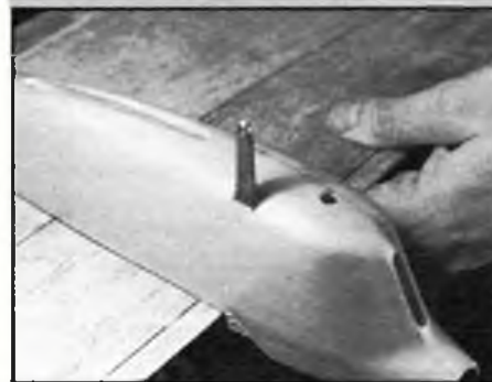
Right shows the Cipolla engine version. This engine is designed for direct fuselage mounting. Six steel pillars are mounted through 1/8 in fibreglass board and the unit bonded in place. Just visible is the edge of the tank which is a snug fit under the rear upper shell. Surgical forceps are a must to install lines, connect tubing and shut off trip.
