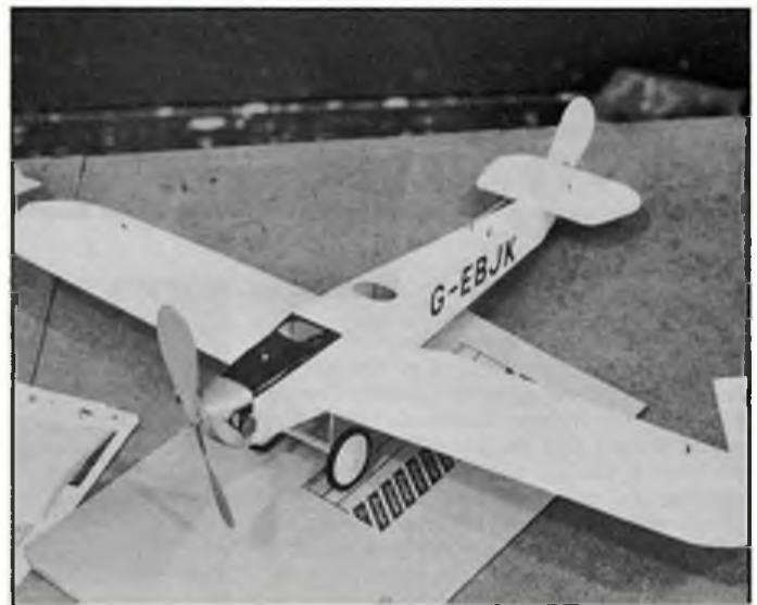
Gordon Hannah's charming Bristol Brownie, 8th in Open Rubber. Wingtip weight is a useful trimming dodge much underrated by non-Indoor flyers.
