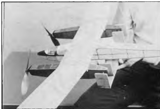
A simple yoke takes the strain out of winding. Long nacelles allow a reasonable amount of rubber and thus good duration.
