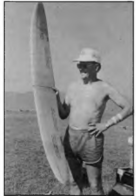
Finland's Ossi Kilpelainen with elliptical dihedral wing, moulded from foam and kevlar - anything is possible with composites...
