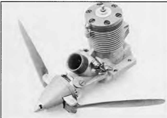
Championship motor - the custom built OMN-25 by Onufrienko, Muhin and Nakonetchny. Note coil spring prop brake behind folding carbon fibre propeller.
