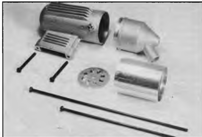
Right: Component parts of the new OS silencer, showing the perforated baffle, extension sleeve and alternative assembly bolts. Below: music is in the ear of the beholder...
