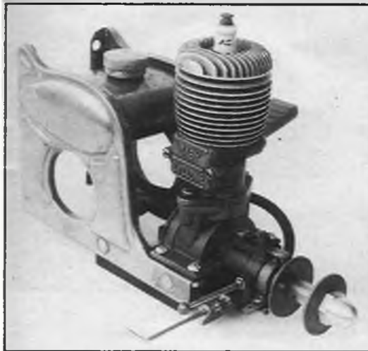
The 6cc Baby Cyclone rotary valve engine, produced from 1935 to challenge the near-monopoly of the Brown Junior. This is the 1937 E model.
