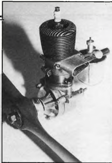
The final's mid-1939 version of the Ohlsson Gold Seal. Bolted-on transfer, exhaust and inlet manifolds on this 9.25cc motor could be a source of leakage and the system was discontinued on later engines.
