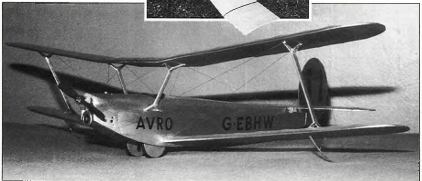
At left: Nautilus II displays its large-area wing and tail. Below: Next in line is this 30in. F/F Avro 558. A Mabuchi 130, geared 3.4:1 and driven by three 50mAH cells will power the as yet untested 3.1/2oz biplane.
