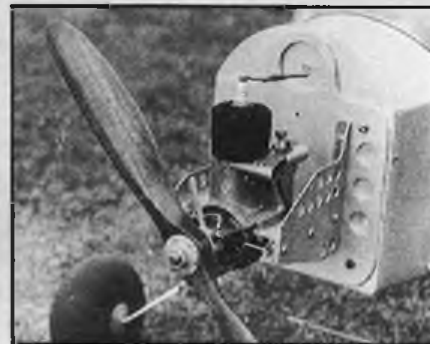
A 1948 Ohlsson and Rice 60 Special sits on a neat mounting in the late John Haggart's Corsaire, a van Wymersch design from the 1938 Zaic Yearbook.
