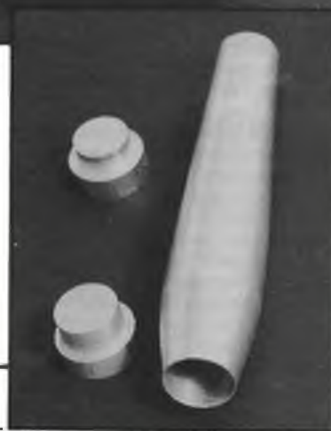
Top: Finished pan, constructed as per Ian's instructions. Irvine .15R is the country's top FAI speed motor. Above: Turned tube, plugs and completed pan. Right: Another view of tube and plugs. Below: Dimensions and angles. All you need to know!
