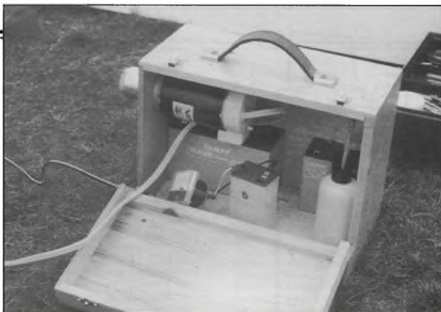
Above: Typical Power accessory box. Neat, simple, relatively light. Starter motor at top left, power sources beneath. Note also fuel, starter accumulator. Tools and spares may also be carried. Left: Jack Allen, flying F1C again at Woodbury Common. Model still being sorted.
