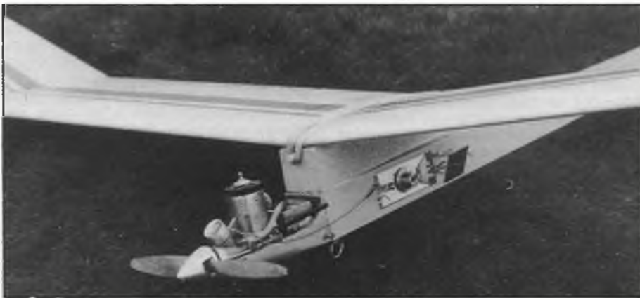
Above: Straightforward and sensible F1C layout – this is Andrew Cordes' model. No cowl; accessible tank (in case of problems) and a Monks timer. Below: Dad Tony Cordes' version incorporates a fairing behind the motor to duct exhaust, and cover tank.
