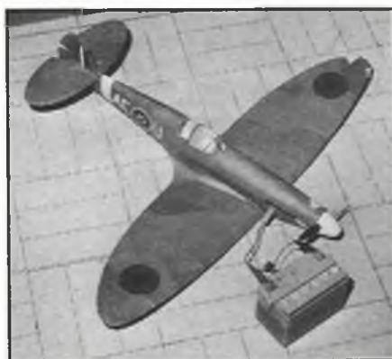
Derek Hardman's fine-flying all-foam Spitfire weighs 70gm for KP power. See text.
