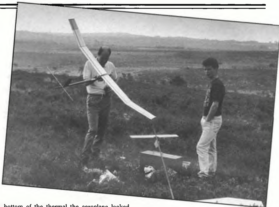
Phil Ball spent FAI Day practicing with new F1C models. Very spectacular with fast climb. Carbon-and-fibre wing features flaps and bunt mechanism. Anthony had a good weekend too with his neat, foam A/2.
