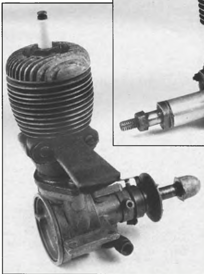
Two interesting motors seen recently – Baby Cyclone at left features seldom-seen exhaust stack; but what's the diesel above? Crankcase looks amateurish, but not the cylinder assembly. Capacity is about 1.5cc. Any ideas?
