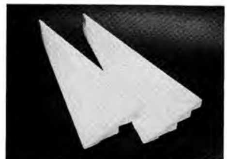
Above: 'fan Block' after the back of the blade has been carved to a flat helical surface.
