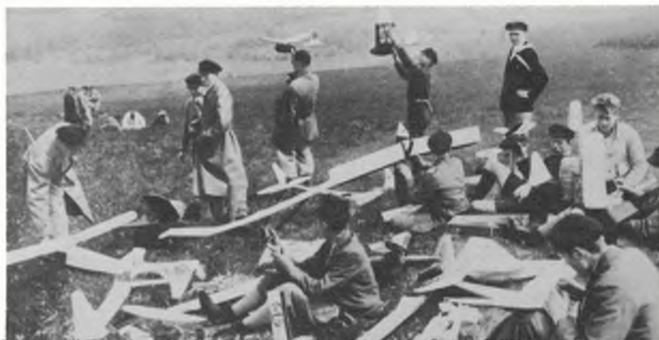
The winged propeller insignia seen on some of these 1920's gliders on the Wasserkuppe indicates that this club was affiliated to 'Ring Deutscher Flieger' whose members were mostly ex-flying personnel from WWI. Some models have stick fuselages but note the tailless machine about to be launched.
