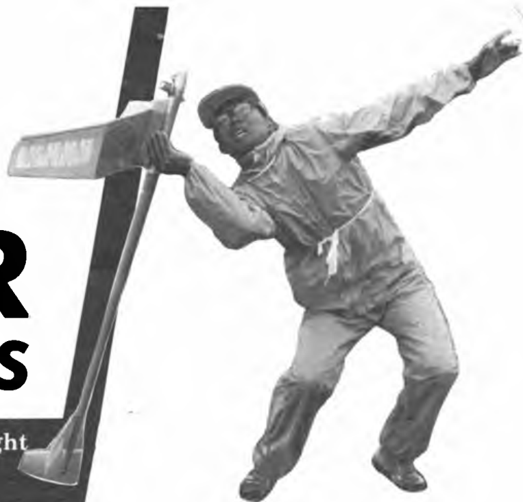
Powerful launch from fifth place Zhijian Cheng - all Chinese models used aluminium surfaced balsa sheet skins on centre panels with built up tips.
