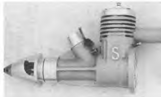
Dave Sugden's handmade F1C motor, note long propshaft, long exhaust, and radial mount. Motor made by lost wax investment casting as described in W/C Symposium Report .
