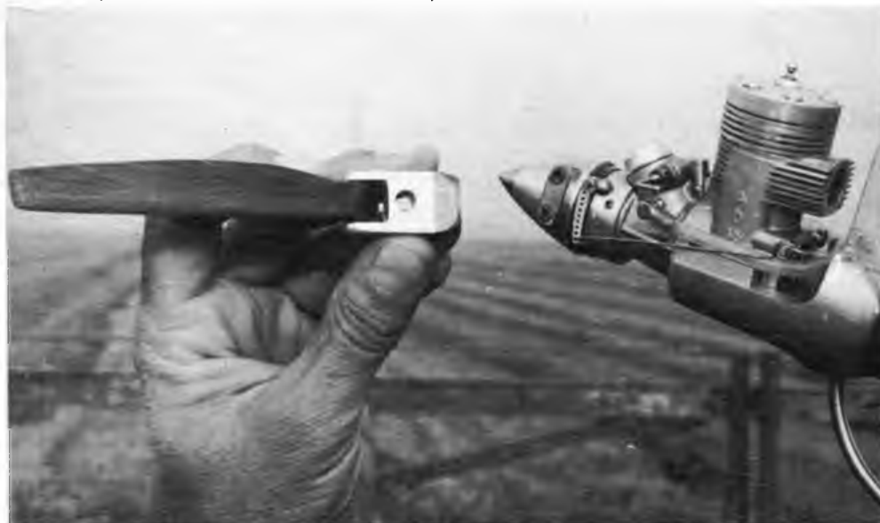
Dave Sugden's handmade F1C motor, note long propshaft, long exhaust, and radial mount. Motor made by lost wax investment casting as described in W/C Symposium Report .
