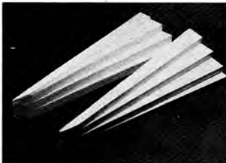
Left and below: propeller blades using 'fanblock' construction — almost ready to carve.
