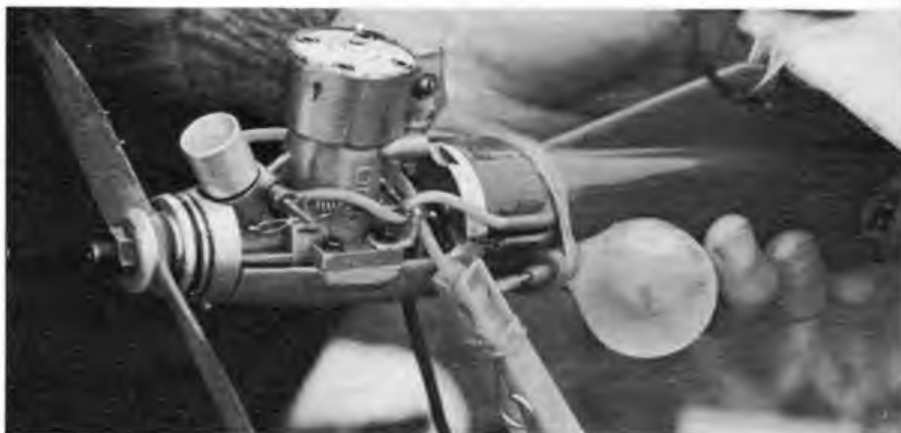
The Ned Kelly of F1C motors, Stuart Sherlock's OPS used head fin insulation to prevent motor cooling during climb to avoid power loss. Motor runs on pacifier and floods off using crankcase pressure metal tank to give advantages of both systems.
