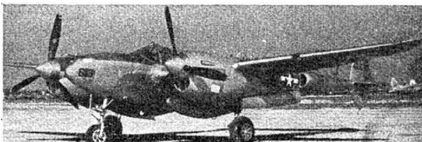
A. T. P. Photo. P-38L: Latest Lightning carries 4,000 lb. bomb-load, has range of 3,000 miles and top speed better than 425 mph.
