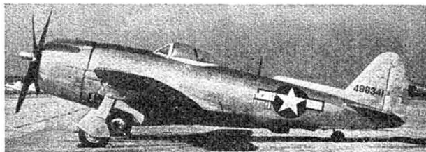
A. T. P. Photo. P-47N: Latest Thunderbolt with redesigned wings, increased range and dorsal fin fillet. Destined for Pacific Zone.
