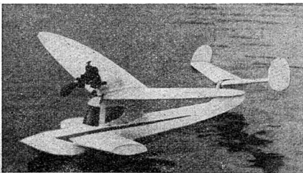
Fig. 2. Col. Bowden's latest flying boat—36" span, suitable for all the smaller engines of 1-1½ c.c. The planked monocoque hull and the flying surfaces are covered with nylon.
