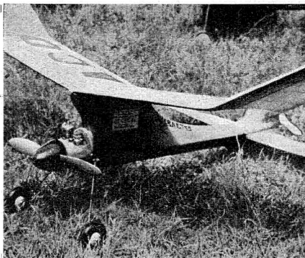
Power model by R. Aubertin of Monaco, seen at the Swiss Internationals. Note large spinner, another example of Continental practice in step with contemporary thought.
