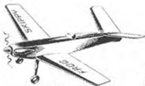
"SKIPPY"— FROG special with a "V" tail for speed and manoeuvrability, 12 in. span.
