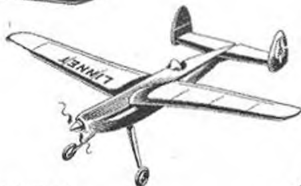
"LINNET"— a super racer, 18 in. span with twin rudders.
