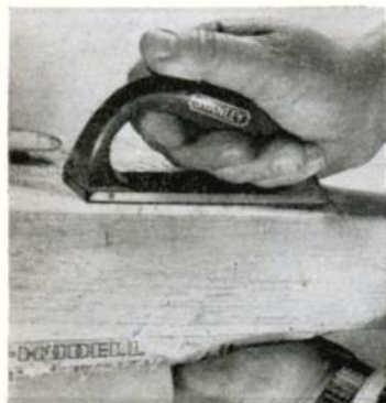
Stanley Jr. Shaper in action on a block of balsa. Is good for roughing out shapes, more useful on glass fibre and hardwood. Blades are replaceable, fit on red plastic handle.
