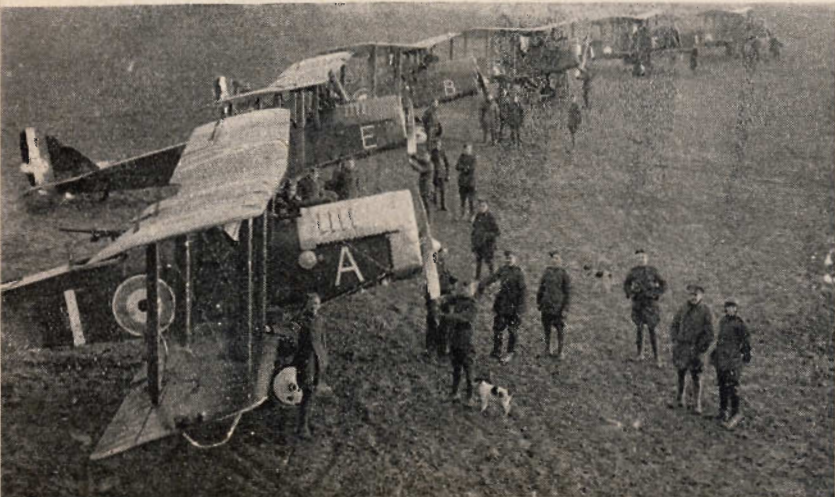
Top view shows a R.A.F. 3A engined D.H.4 of 18 Sqn. Note bomb racks under wings and forward pilots cockpit. I.W.M. Photo. Q11672. Left: B.H.P. engined versions of 27 Sqn. "E" is only one with extension to exhaust. Note polished cowl on "A" and high Scarff rings. I.W.M. photo Q12015
