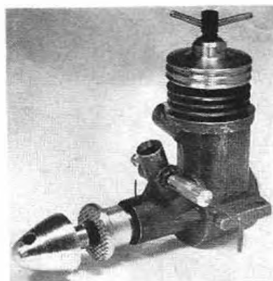
Two views of the Soviet 'Veterok' 1.5 c.c. diesel, an example of the small general-purpose model engine available to Russian modelers.
