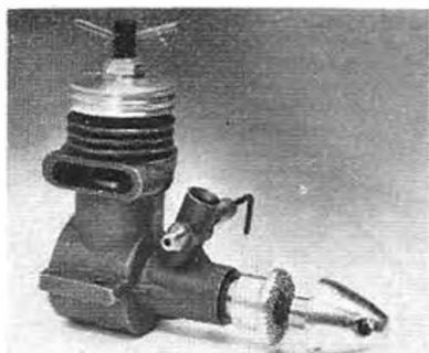
Two views of the Soviet 'Veterok' 1.5 c.c. diesel, an example of the small general-purpose model engine available to Russian modelers.
