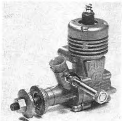
Without silencer the Fuji weighs 4 ounces. Heading illustrates the pivoted plate on silencer for starting.
