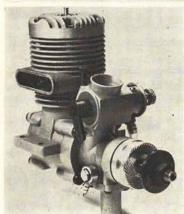
the Rossi 15. To achieve this, the piston has been made very thin with a 15 thou. skirt and 30 thou. head and the oval-section conrod shank is actually hollow. The complete piston, rod and pin assembly weighs only 6 grammes. The piston is flat-crowned and deflectorless and the gudgeon-pin is placed high in the piston in order to reduce conrod angularity.
