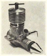
advertised in the May issue of Aeromodeller. Selling at £4.95, the Sokol is no Oliver-Tiger, either performance or quality wise, but its design follows a well-proved and familiar pattern for 'sport' type diesels. In other words, it is a plain bearing, beam-mount motor with radial cylinder porting and shaft rotary-valve.
