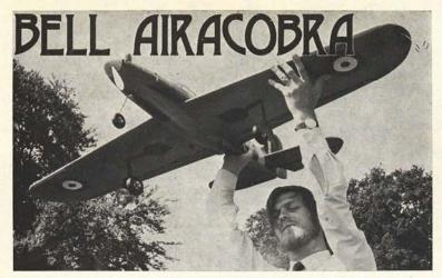
a 60 in. span semiscale control line stunter, featuring a detachable wing, for use with 0.35-0.40 cu. in. motors, designed by ROBIN WOODHEAD
