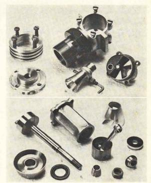
More parts of the Lopatenko glow engine. Crankshaft is very long and slim, being composed of four parts. Conrod is hollow in effort to reduce reciprocating weights.
