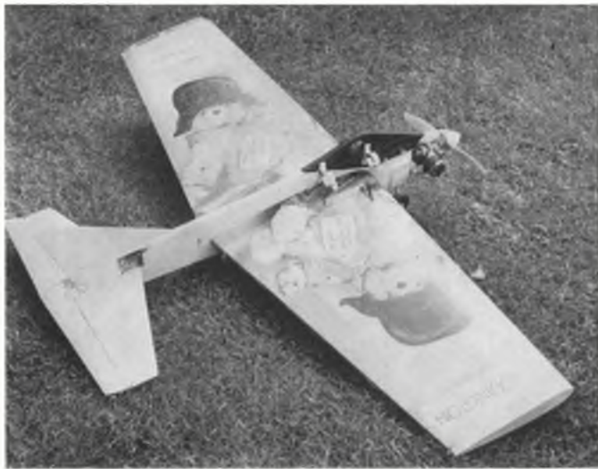
The Wembley 'Aerostar' - the prototype for which was designed, built and flown in just two days. Note the free-flight timer below fin to deploy different colour streamers and Terry clips on fuselage to hold smoke canister. Sullivan R/C clunk tanks used - made checking fuel levels very easy.
