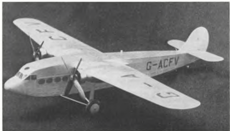
Our columnist's Avro 642, which spans 26in. and weighs 90 grams is equipped with a pair of Telco CO 2 motors - the tanks being mounted in the fuselage. Converted from a rubber powered model, it features turned aluminium cowlings and working suspension.
