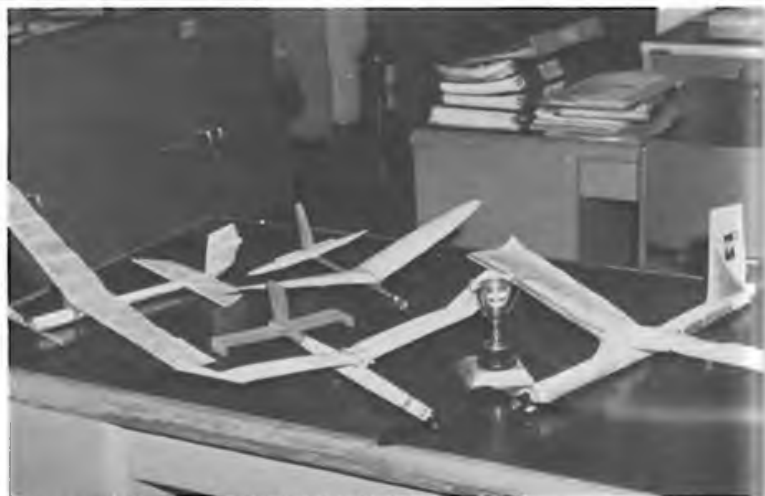
Top left: 'A' frame pusher in card! Span 42cm, length 44cm, 42 grammes with 13cm propellers in bent plywood. Total power 18 office elastic bands giving a long powered glide of about 70 feet.
