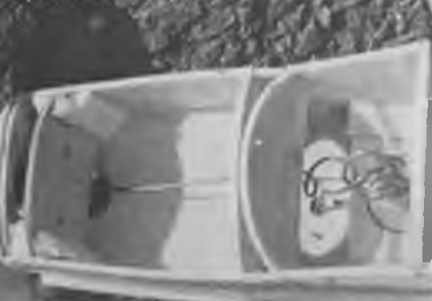
Below, VERON Bolkow Junior Kwik—Built kit. Tapes mounted on 1/16in ply bulkhead tank fills further back to prevent nose heaviness.
