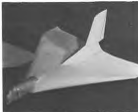
Top left: 'A' frame pusher in card! Span 42cm, length 44cm, 42 grammes with 13cm propellers in bent plywood. Total power 18 office elastic bands giving a long powered glide of about 70 feet.
