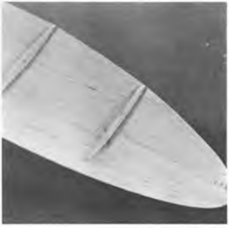
Above, view of underside of wing shows simple ribs which keep top sheet to aerofoil shape behind triangular leading section.
