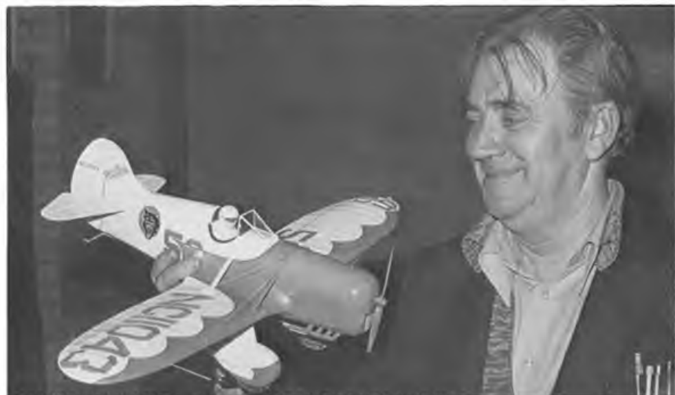
Below: Bernard Sexton seems pleased after the first test flights of his Gee-Bee Model 'D' to 1/12th scale (28in span) for electric RTP. Vivid blue and white scheme makes an attractive subject but model is to be re-engined with a larger motor and prop
