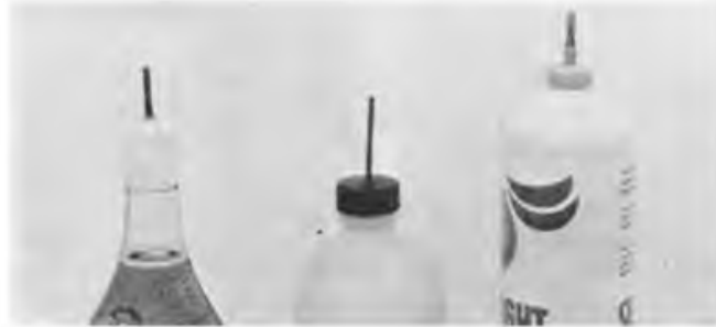
Left. Assorted plastic squeeze bottles suitably modified for filling fuel tanks are much better than the metal cans in which the fuel is sold
