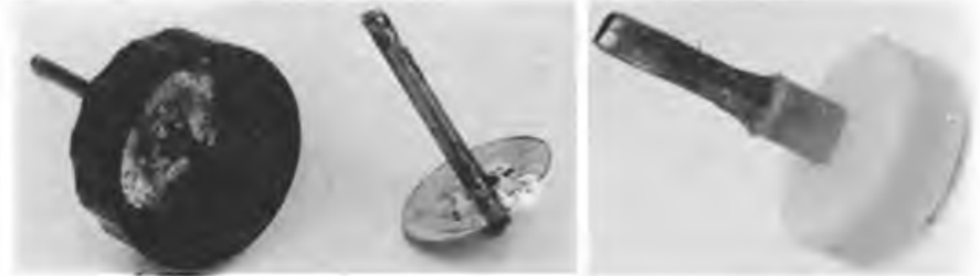
Below. 1/8 inch dia brass tube soldered to tinplate disc before fitting inside brittle plastic top.
