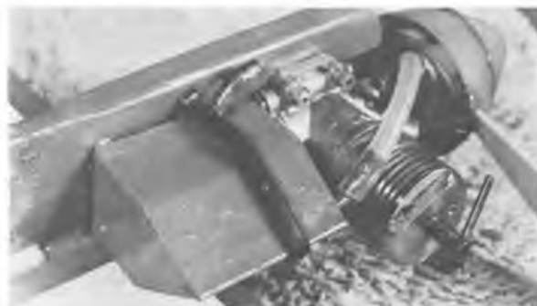
Two simple methods of fixing fuel tanks to the side of profile fuselage models. Left, rubber fuel tube strap retained by threads of 6BA bolts. Right, tinplate strap cut from old can, can be soldered to tank.
