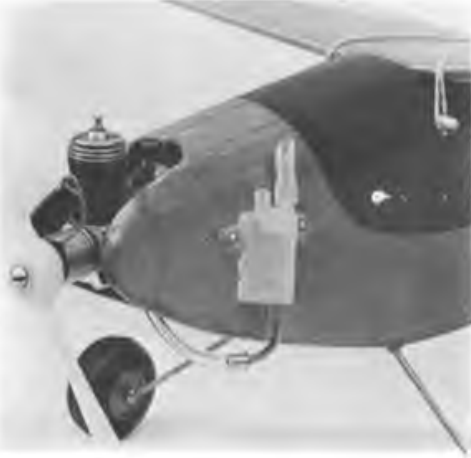
Below, nose details, standard commercial graduated tank cut down and fitted with angled brass pipe to give visual fuel indication.
