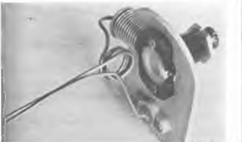
Telco motor and filler both mounted on ply former ready for installation into a HUMBROL Racer.
