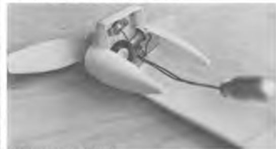
Motor and filler tested for fit inside VAC formed cowling to check propeller clearance. This power module can later be fitted to other models.
