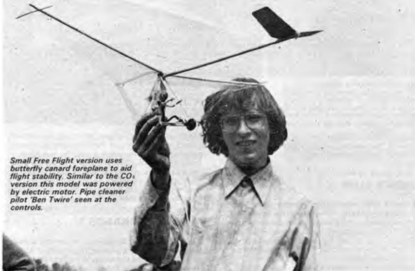
*Small Free Flight version uses butterfly canard foreplane to aid flight stability. Similar to the CO<sub>2</sub> version this model was powered by electric motor. Pipe cleaner pilot 'Ben Twire' seen at the controls.*
