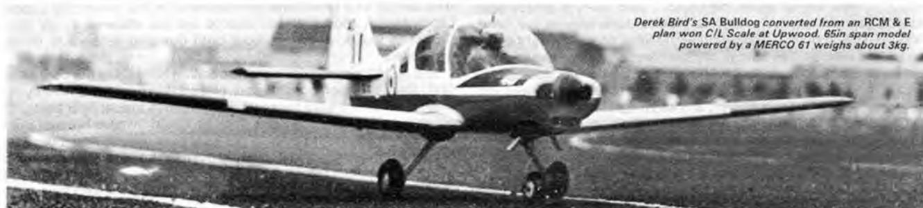
*Derek Bird's SA Bulldog converted from an RCM & E plan won C/L Scale at Upwood. 65in span model powered by a MERC0 61 weighs about 3kg.*
