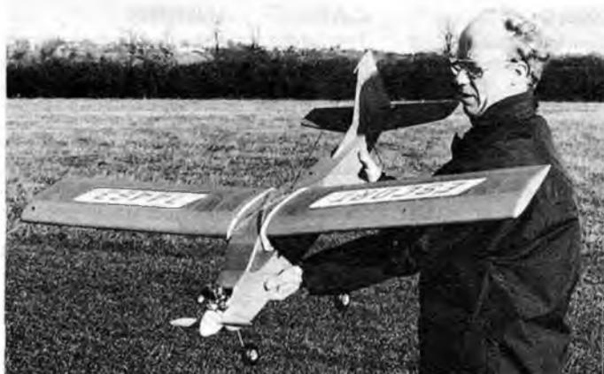
Left: Stan Rose constructed this Galaxy Models Escort powered by trusty Enya 19 specifically for the R/C Sport Flyer series. Although the all-balsa built up construction took a little longer to assemble than other "prefabricated" kits, the Escort nonetheless proved an ideal R/C trainer and is definitely the type of kit for the modeller who really enjoys a bit of building.
