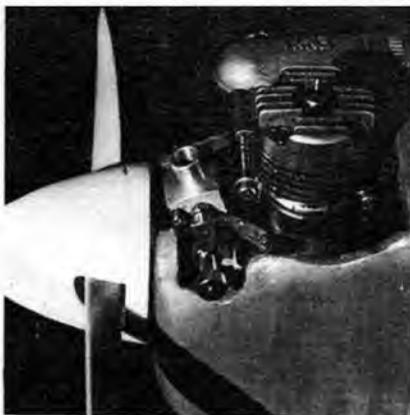
Left: Close up detail of Enya 19 fitted with mandatory silencer neatly installed in the nose of the Galaxy Escort.
