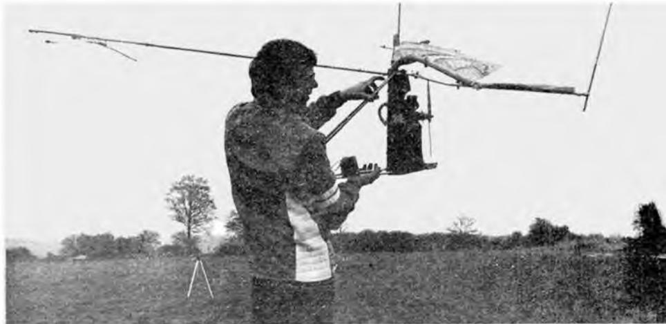
Above: Side view of huge 4 metre span machine shows leading edge tube curved to correspond with billow in wingsail
