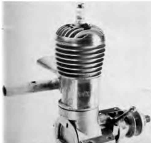
Left: the Gwin-Aero with tank/needle-valve assembly removed. Note lack of assembly screws. All-steel cylinder had integral head and was threaded to crankcase, as was backplate.
