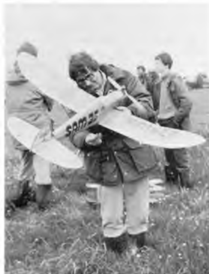
SAM Treasurer Peter Michel with his Peerless Panther one of the first successful low-wing power models to be kitted. It was powered in its original form in 1940 by spark ignition engines like the Ohlsson 23.
