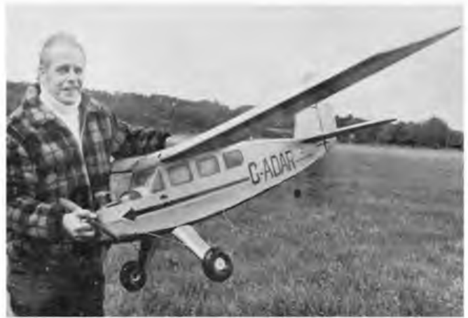
"All Weather Pat!" The OS60 powered Vulcan with its builder. This fine pre-war design by the late D. A. Russell looks and feels like a real aeroplane. Originally in 1939 it was powered by a 9.2cc Dennyrite "Airstream Deluxe" petrol engine.
