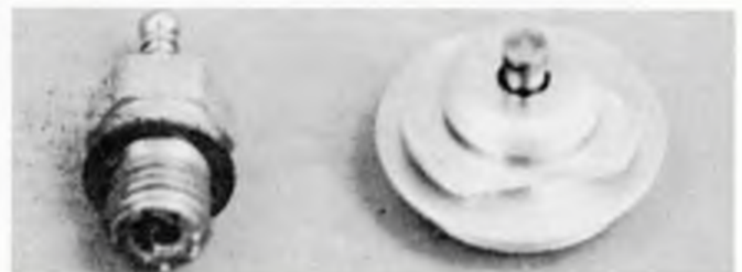
Left: various commercial glow plug clips and below an individual plug on the left with an integral cylinder head and plug on the right.
