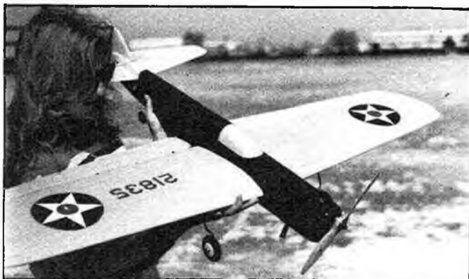
Paul Smith's renovated Midwest PT-19 built in 1964. Foam canopy and turtle deck replaces the original wood blocks and cockpit detail.
