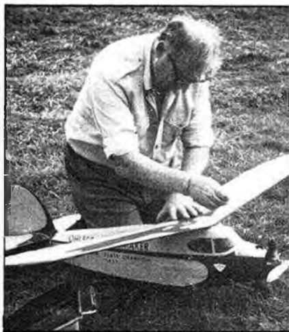
Above centre: Keith Harris with his Ohlsson Pacemaker powered by Mechanair 5.9cc petrol engine. Model is finished in the original Ohlsson colour scheme; good on you. Keith! Left: the writer's Kollbrik powered by Amco .87Mkl diesel. This design is still available from the MAP Plans Service as PET/245X. The 31 1/2 in. wingspan model is a real challenge and can be tricky to trim well. Below right: Mr. Simeon G. Bull of Canterbury sends this nice study of his Jackdaw II coming in 'dead-stick' over the proverbial long grass on its first day out.
