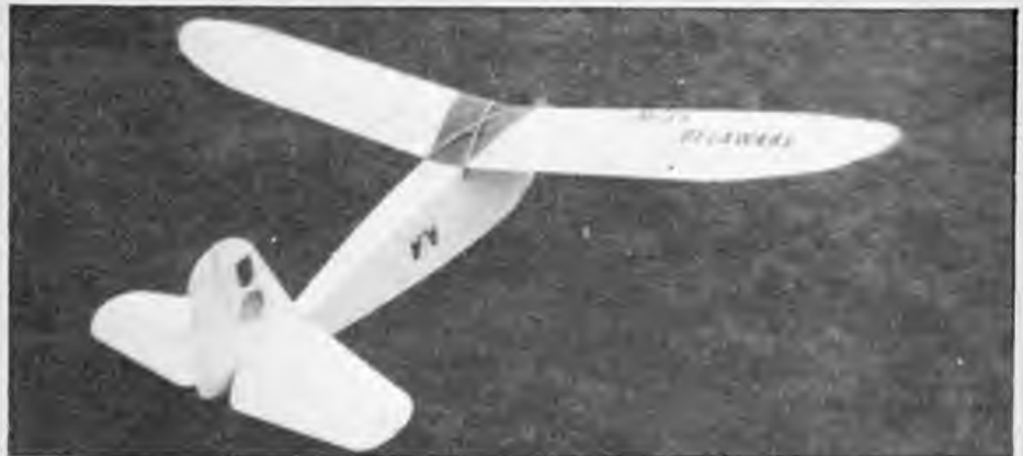
Above, Mike Parrott of Bletchley built this Miss Delaware, an 37in. span Stephan Kowalik design which won the Junior Motors Trophy in 1936. Power here is a Merco 61, with Fleet R/C on three functions. Model reportedly a very pleasant flier. Below: a common sight at meetings in the immediate post-war era, many modellers travelled by bicycle or motorbike carrying their models thus! Who will be first to tell us who, where, when and identify the model?
