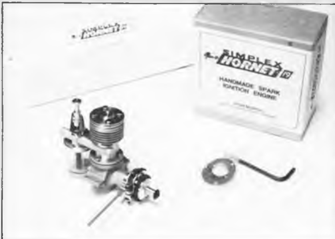
Below John Morrill's Hornet 19 sideport ignition engine, production of which is well into the second batch - see text for details.
