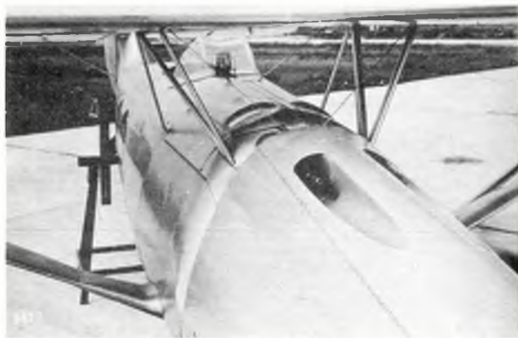
Cockpits in the thirties weren't neat, lined or designed for comfort. The Stösser carried the impression of being a fighter, with spade control column, cast heel plates and a Revi sight in the windshield. Centre: the Heine fixed pitch prop and elegant cowling were particular Stösser characteristics. Above: starter handle in position, and filler cap removed in this rear cowl angle which also shows the neat strut fairing for the u/c. Below left: inside the cowl was no less neat. Engine bearers, gun faired crankcase and tidy installation are typically precise. Below: the sleek fuselage, gun troughs, and clean cabane strutting.
