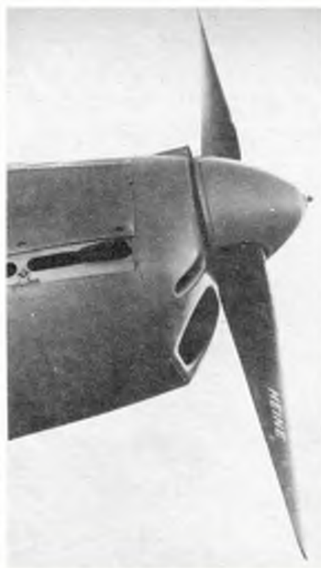
Cockpits in the thirties weren't neat, lined or designed for comfort. The Stösser carried the impression of being a fighter, with spade control column, cast heel plates and a Revi sight in the windshield. Centre: the Heine fixed pitch prop and elegant cowling were particular Stösser characteristics. Above: starter handle in position, and filler cap removed in this rear cowl angle which also shows the neat strut fairing for the u/c. Below left: inside the cowl was no less neat. Engine bearers, gun faired crankcase and tidy installation are typically precise. Below: the sleek fuselage, gun troughs, and clean cabane strutting.
