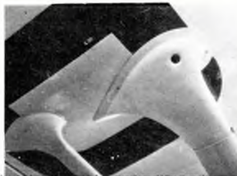
Tailplane forward of the large rudder was a design 'signature' adapted from Albatros. The endplates appeared in subsequent Fw designs. Above: the small divebrake on the centre section, shown open. Right: cockpit side flap for access carried instruction panels on the inside and on 'KNI', the Gilmore Lion sponsorship trademark was outside. Below: the shaped military style seat and height control arm, close up of wing strut fairings, undercarriage oleo and torque links without the trousers shroud.
