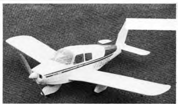
Ian Peacock's Piper 'Cherokee' converted to electric power, only modifications needed were in the mounting of motor and batteries. Note motor slightly off centre - see text.
