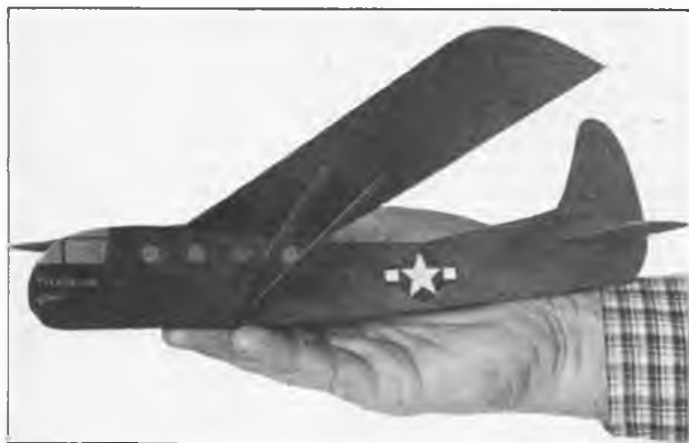
This view of the Waco 'Hadrian' clearly shows the simplicity of construction - just take care with those wing struts! A felt tip pen and a few decals (transfers) will make all the difference to the final appearance.
