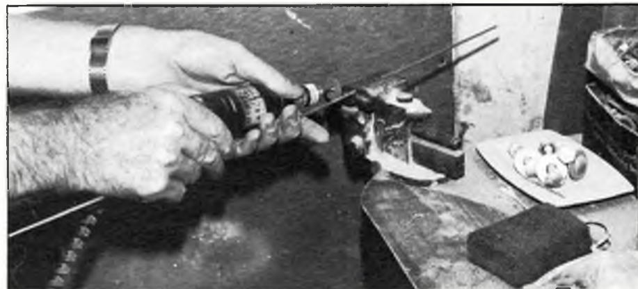
The uses of hand held 'drill' are almost boundless. Above, using a carborundum disc to cut heavy gauge piano wire. Right, abrasive tools in many shapes help finishing awkward shapes, this cowling would be much more difficult to 'clean up' with just a file!
