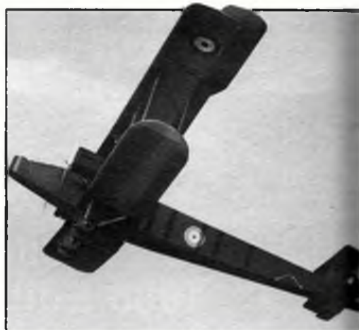
Above, this fine shot of Bill Dennis' free flight Handley Page 0/400 was taken by Rex Oldridge. It is powered by two Mills .75s with a common cut-out. Lines on the fuselage are shadows of the wing struts.
