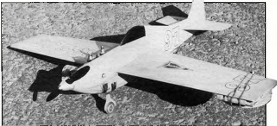
"Ol Blue 72" (Class 2 Goodyear) with its squared off tips and straight taper wing makes it easy to build - join the winners build one from our plans overleaf...
