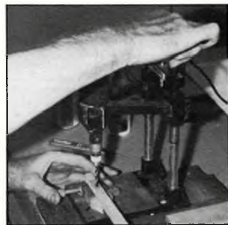
Above, probably the most sensible way yet of cutting slots for fuselage stringers, using abrasive disc(s) in a mini-drill. Right, another variant, this time from Mini Craft of a mini-drill stand.
