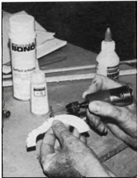
Above, probably the most sensible way yet of cutting slots for fuselage stringers, using abrasive disc(s) in a mini-drill. Right, another variant, this time from Mini Craft of a mini-drill stand.
