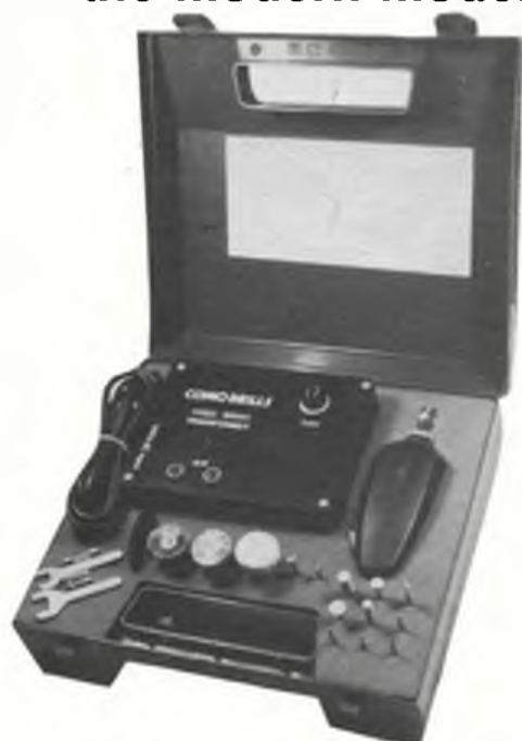
Left, like other manufacturers of mini power tools, Como too, have several 'sets' that include fixed or variable power supplies and a variety of useful tools.
