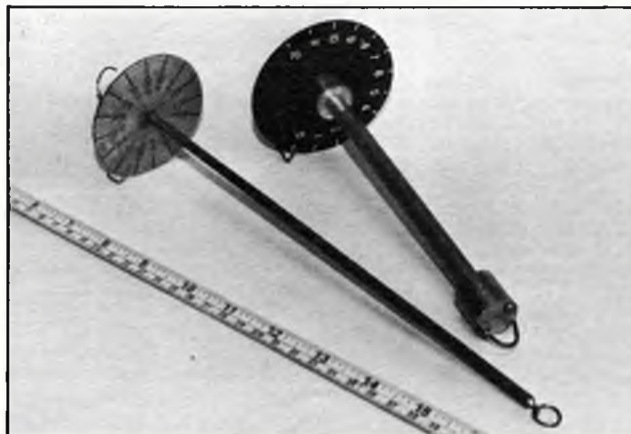
Left, the Coupe d'Hiver Torque meter reading up to 40oz/in - left. Compared with the Woodhouse unit for larger loads on the right. Both worth their weight in rubber!
