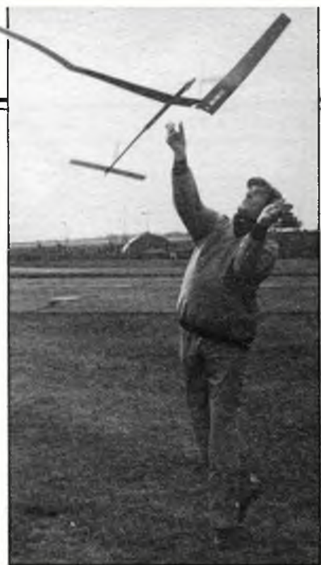
P. Gaunt in all manner of trouble at the Grantham G.P. after quite a gentle launch. His designs have very thin solid wings and its the first one to go like this. Note the reverse load flexing the starboard tip down now all the torque is trying to twist the fuselage. (Grantham G.P.)
