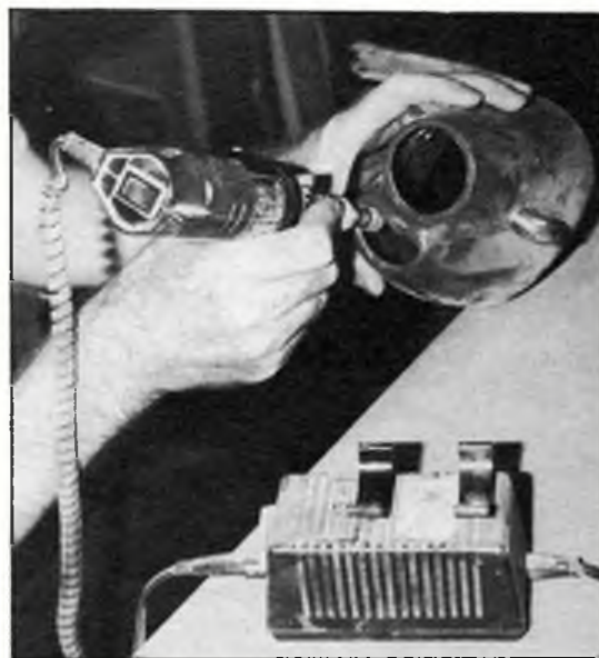
The uses of hand held 'drill' are almost boundless. Above, using a carborundum disc to cut heavy gauge piano wire. Right, abrasive tools in many shapes help finishing awkward shapes, this cowling would be much more difficult to 'clean up' with just a file!
