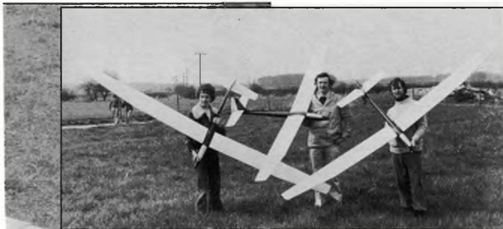
Main photo, left: The author's Aeolian, designed in 1976, was of 12ft. wingspan and 8oz/sq ft loading. Apart from the root airbrakes, it is a typical model of the period. Above: Derek Martin designed the Cadenza P80 in 1980. These three prototypes won many contests, including the Nationals, in the hands of R.R. clubmen. Below: A collection of typical open models from 1977, showing the then-common 'traditional' structures.
