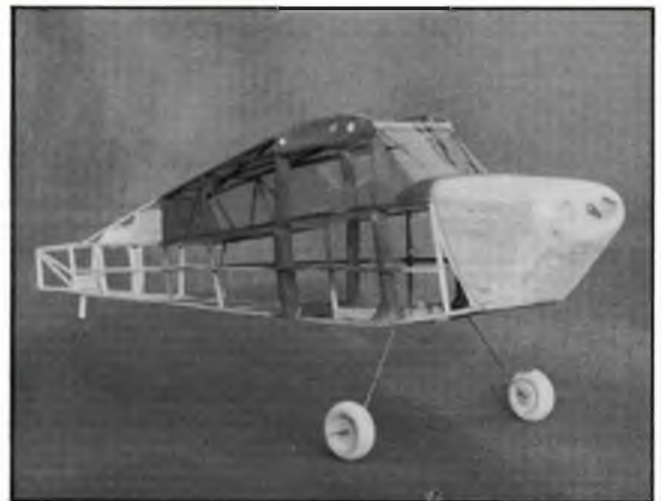
Above: The L-6 is an attractive subject. John chose to finish his prototype in pre-war U.S. trainer colours, i.e. blue fuselage and fin, with red and white rudder stripes, and yellow wings and tail. Right: The basic fuselage structure. Cowling is easily fashioned from block or laminations of sheet.
