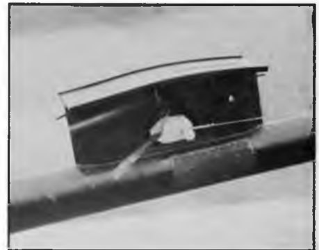
Neat Tomy timer installation in Russell Peers' Head Beagle F1B (last month's Free Flight Scene drawing).
