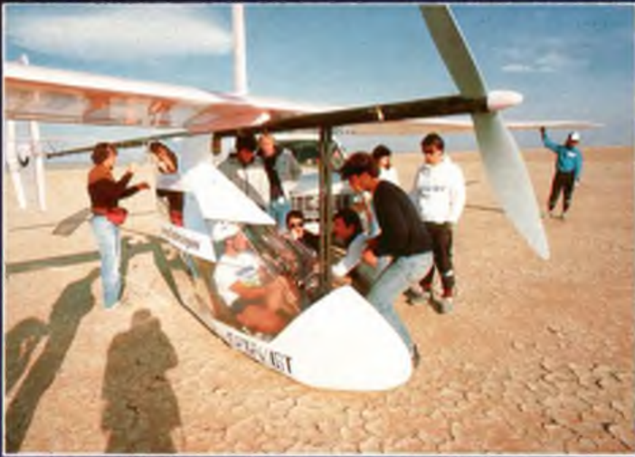
L to R: 'How did it go' — Post flight checks by the Flight Directors and Engineers logged every detail. At this stage the drive shaft aerodynamic fairing is not fitted. Who played with the Daedalus name stickers we wonder! (Mike Smith photo). Next: Preparing the mainspar for assembly — not so far removed from aeromodelling techniques (Peggy Scott). Next: The Imported Hangar at Hørsholm proved more difficult to erect than the three HPAs! (John McIntyre). End photo typifies the continuous training programme for the five pilots on the project. Road work plus the simulator kept fitness at peak (Steve Finberg).
