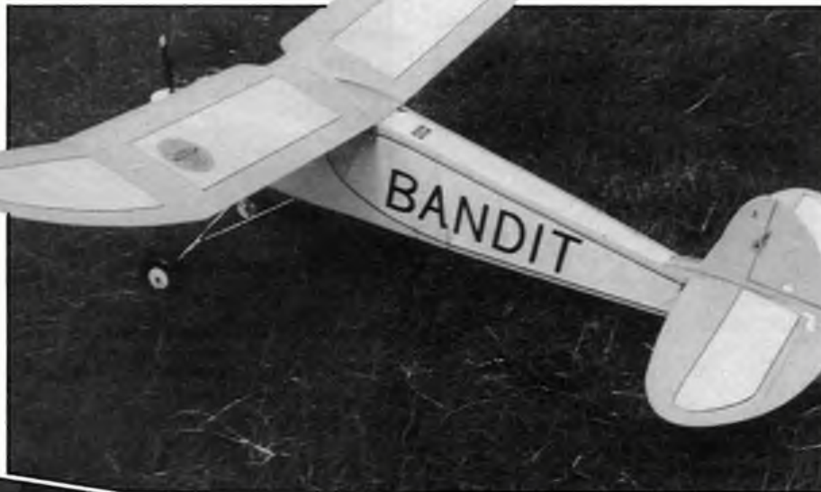
Above: You too can have a finish like this! Ken Tansley's double-sized Keil Kraft Bandit from Balsa Cabin plans is Merco 49 powered and has Fleet R/C gear. Undercarriage is beefed-up. Secrets of neat nylon covering in text. Left: US model aviation historian Walt Grigg sent us this shot of his original Rigby Swallow in the box! Total cost from manufacturers, the Vase Press Ltd, Thrapston, Kettering was 2/6d! Below: A Joe Ott box from the Whitman range, beautifully printed in five colours. Pic from Walt Grigg, who enjoyed our tribute to Ott in last December's Vintage Corner.
