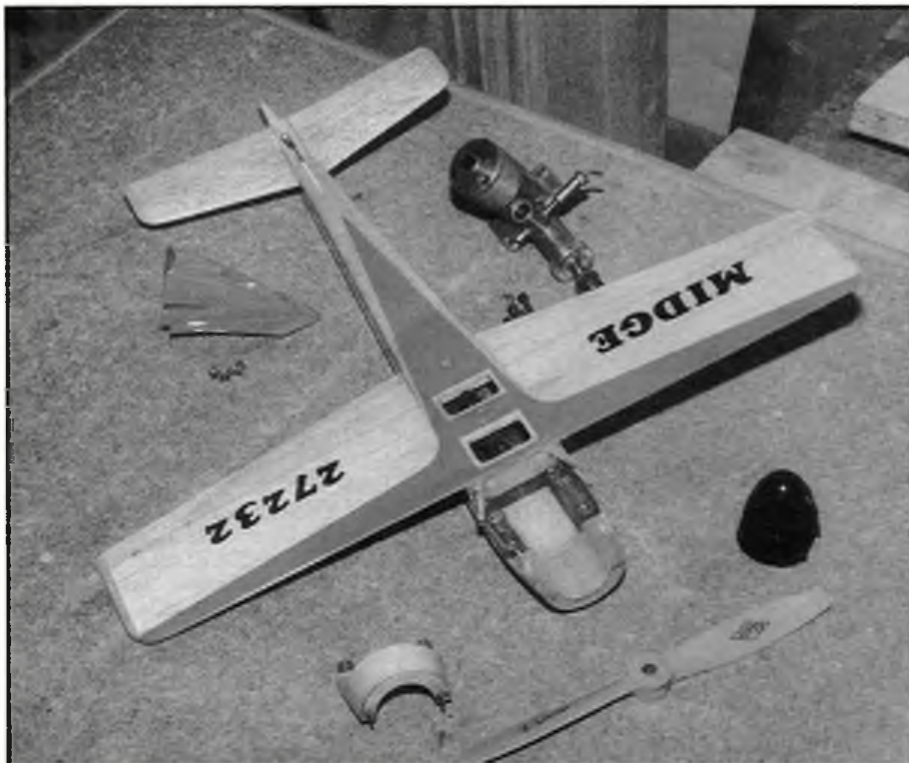
Engine out - and the removable rear cowl reveals bellcrank through fretted wing centre section.
