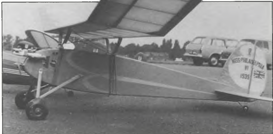
Noel Barker's replica of pioneer Maxwell Bassett's eight-foot parasol Miss Philadelphia. Because of present-day materials and building techniques, replicas are often heavier than the original models. Bassett's covered with bamboo paper tipped the scales at 4lb. ready to fly. The writer's version (nylon covered) is one pound heavier.
