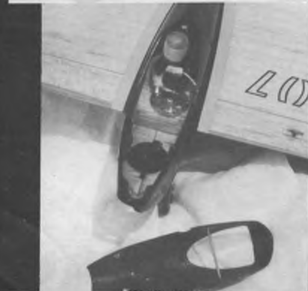
Above: The carbon fibre/epoxy moulding by Patrick Constant for Team Racers. Bosses and ribs are moulded in; note cooling and exhaust duct, top cowl and undercarriage box. Left: Business end of complete model.
