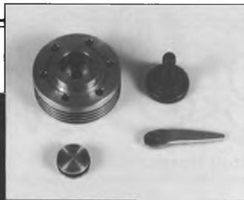
Left and top: Barry Shaw's diesel home-conversion of the OS Max 40FP. Simple chamber in head accepts alloy contra-piston and O-ring. R/C throttle is fixed in fully-open position when motor runs as diesel.
