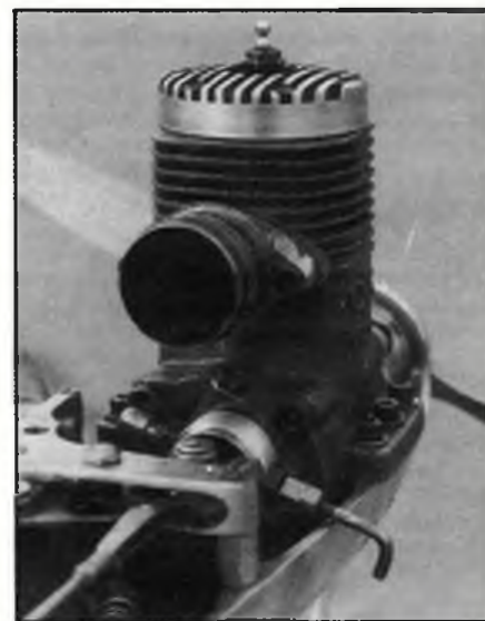
Heading and above: Two views of the most powerful Speed motor yet; Ken Morrissey's OS Max 61V - a converted marine engine. Note sub-spar and bellcrank assembly, as detailed in text.
