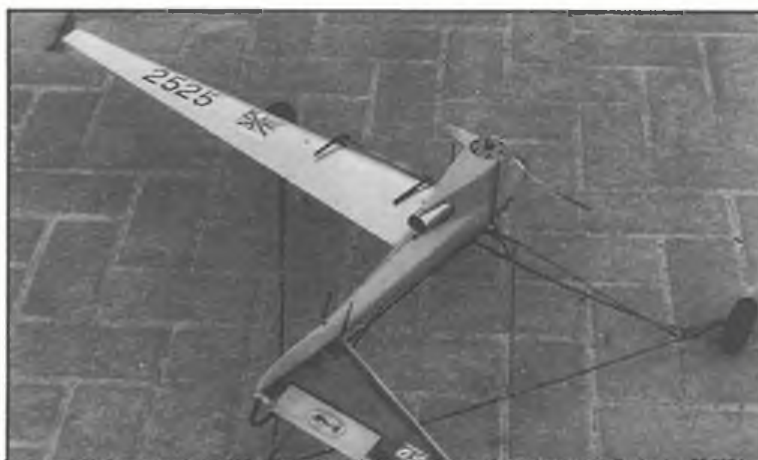
Details of tough wing sub-spar and 'button' line connectors.
