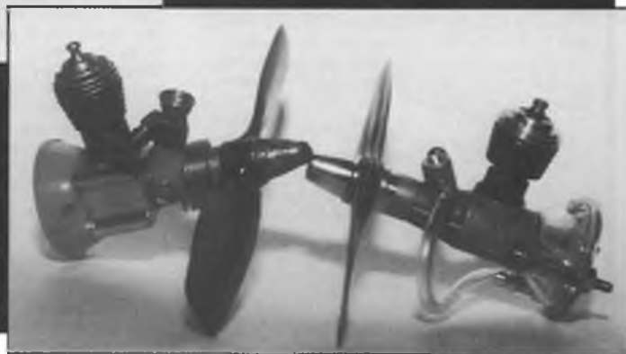
Right: Small-glow duo. Well-known Cox .010 (0.16cc) faces the even smaller T Wasp of 0.098cc.
