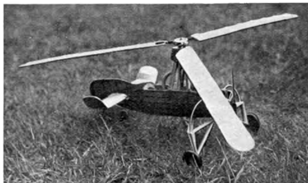
Mr. Fieldgate's (Wembley and District) fine autogiro. Has fully hinged blades which are controlled from cockpit. It is built entirely from balsa.
