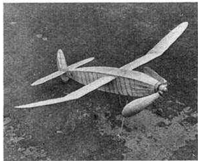
P. E. KUNISS (Denmark)—45½ in. span shoulder wing streamlined slabsider, section Gottingen 359, double-bladed folder and pop-up tail D/T.
