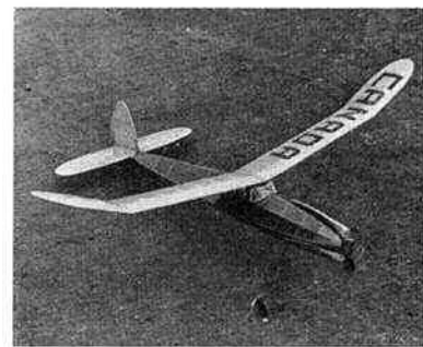
R. LEQUVER (Canada) —"Flying Cloud," 43 in. span streamlined cabin slabsider, diamond rear fuselage and polysided front, double-bladed folder.
