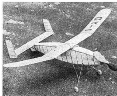
P. B. CHRISTIANSEN (Denmark)—41½ in. span parasol slabsider with a double-bladed free-wheeling prop, short fuselage and large twin fins.
