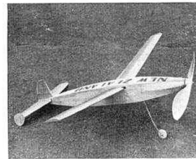
A. MACDONALD (New Zealand)—Shoulder wing streamlined slabsider, double-bladed free-wheeler, and single fin with tailplane endplate sub-fins.
